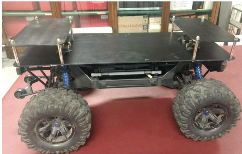
**Figure 1-4.** Vehicle with its tradition made fiberglass support plate.
