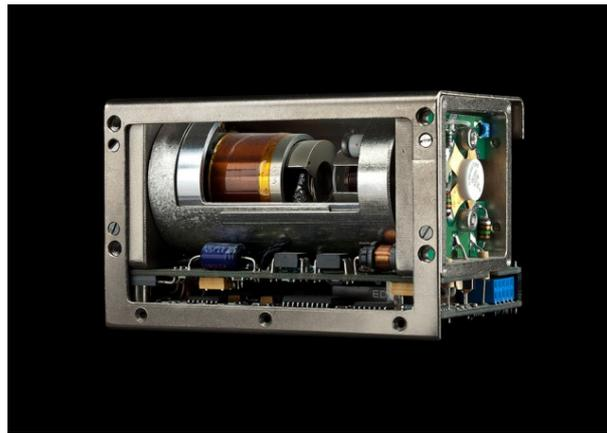
**Figure 1.1:** Rb atomic clock, Temex Neuchâtel Time S.A., 1995 in collection of the Le Locle museum in Switzerland.
