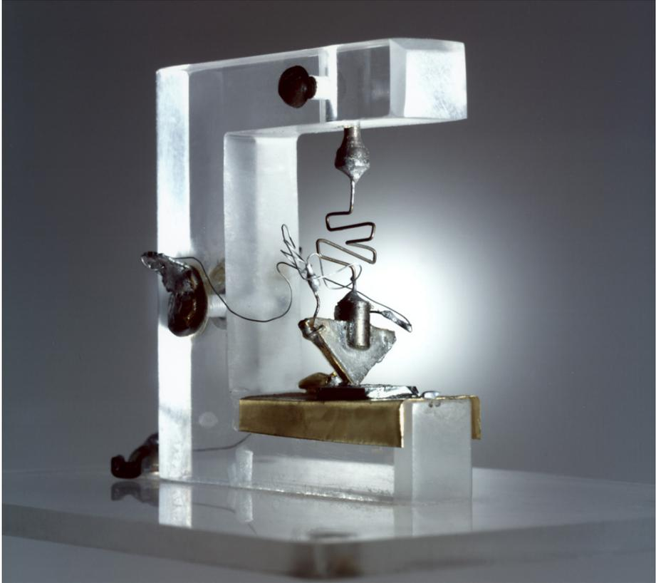
Figure 1.2. The first Germanium bipolar transistor [1].
