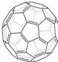
Figure 2.1. Structural illustration of a Fullerene [19].
