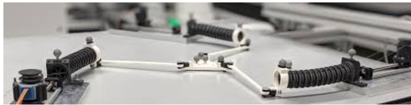
(c) Tendon Actuated Planar Parallel Continuum Robot, image from [16]
