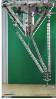
(a) Continuum version of the Delta robot, (b) Continuum Stewart-Gough robot, image from [25] from [17]
