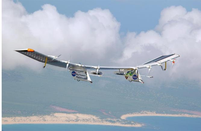
**Figure 2.7:** An example of aerodynamic platform used as a HAPS [49]
