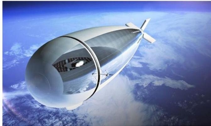
**Figure 2.6:** An example of airship used as a HAPS [48]
