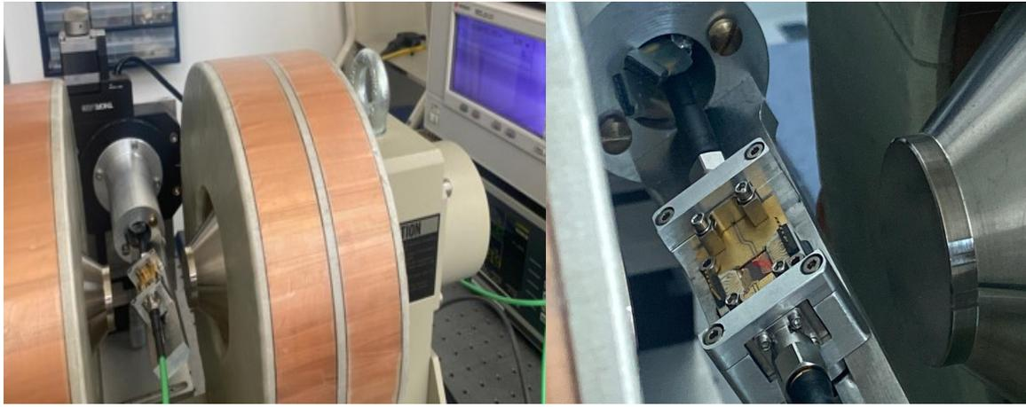
**Figure 3.10:** Experimental setup. Left: the sample holder, attached on a motorized rotation axis, is centered in the middle of the Helmholtz coils magnet. Green microwave cables connect it to the microwave generator and spectrum analyzer. Right: zoom on the PCB where CPW lines can be seen connecting the microwave cable to the on chip device.
