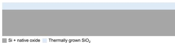
The starting substrate is a 500  $\mu\text{m}$  thick Si one on top of which 500 nm of  $\text{SiO}_2$  are thermally grown.
