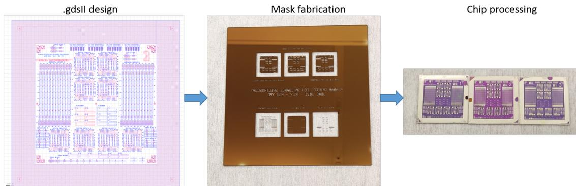
Figure 4.32: Schematic representation of the process flow of the planar devices fabrication, passing first from the design and the mask realization for then arriving to the actual processing of the chips.
