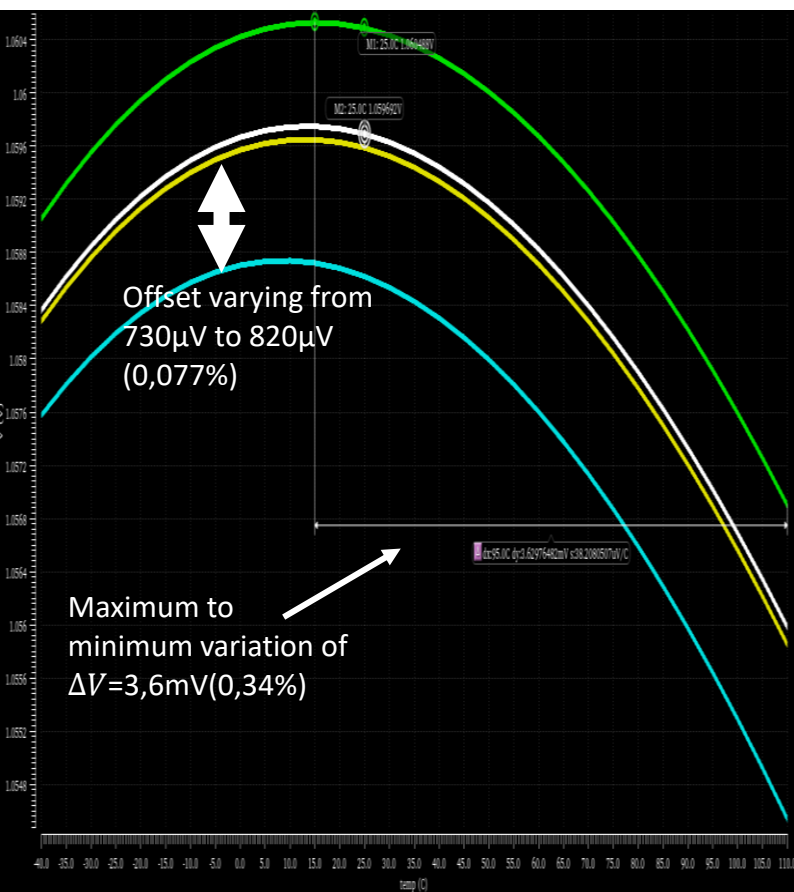
Figure 35: V_{ref} as function of temperature. Blue : new version's layout extraction, yellow : schematic without parasitic, white : schematic with parasitics and green : old version's layout extraction
