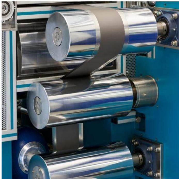
*Figura 2.9 - Roll-to-roll process FAAM (Carlo Novarese - FAAM)*
