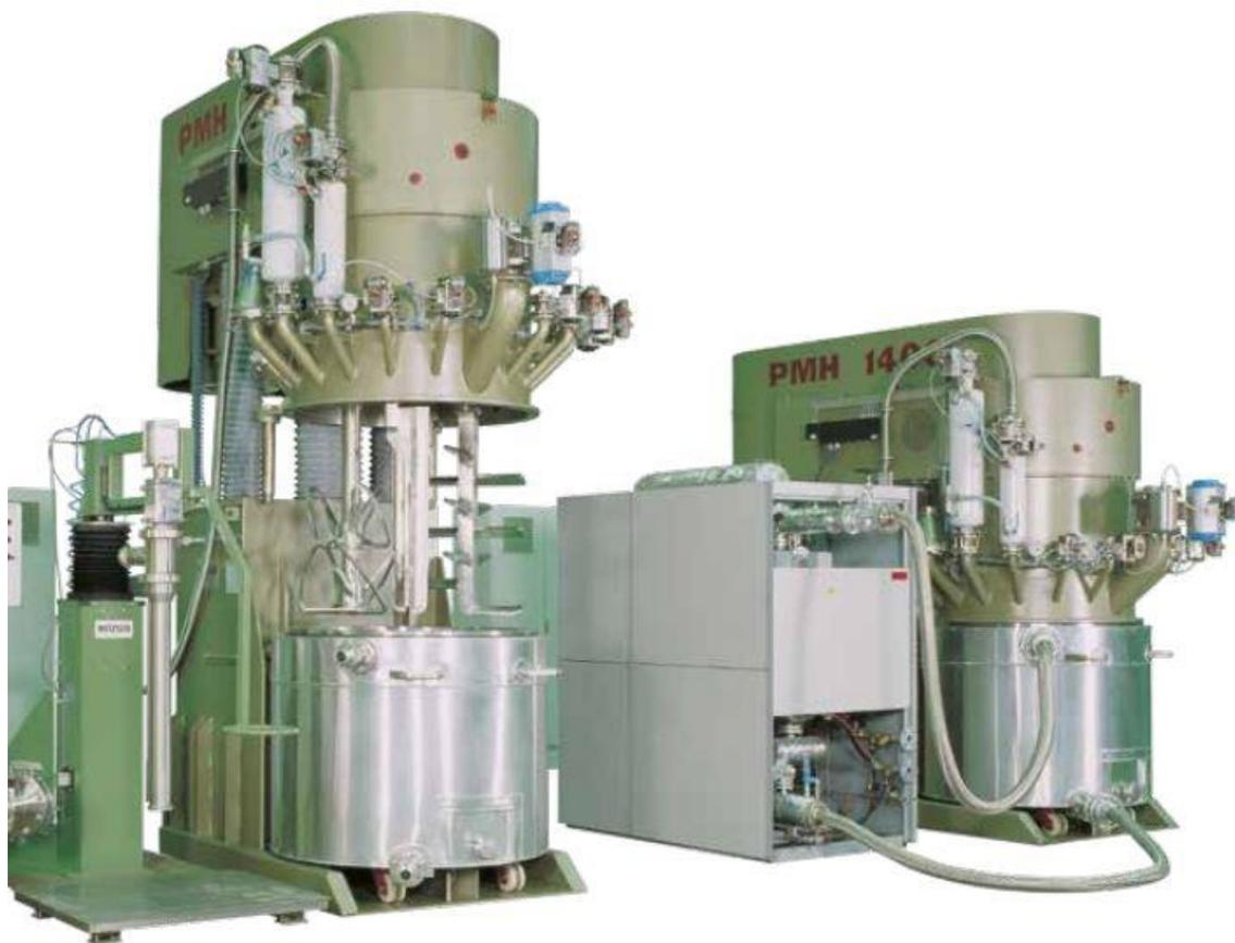
Figura 2.1 - PMH Planetary Mixing e Kneading Machine - NETZSCH (NETZSCH)
