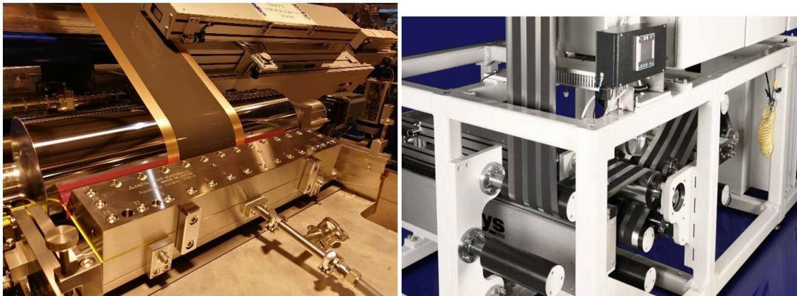
Figura 2.4 - Coating continuo (sx) e coating discontinuo (dx) (Carlo Novarese - FAAM)
