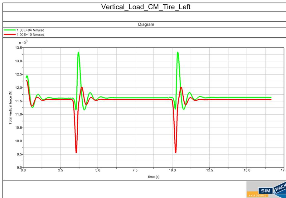
**Figure 4.13:** Influence of the maximum and minimum stiffness parameter on the vertical load (CM)
