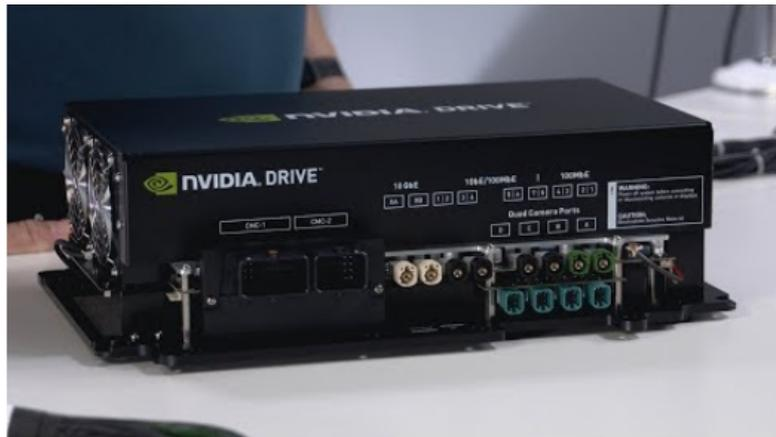
Figure 2.1: NVIDIA DRIVE AGX Developer Kit
