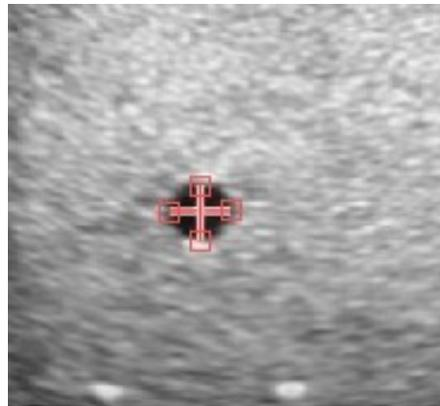
Figure 3.14. Example of horizontal and vertical diameters measurement on one anechoic cylinder on an image (detail).
