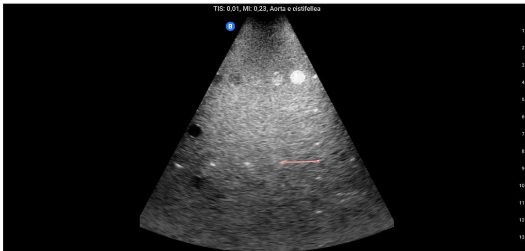
Figure 3.10. Example of horizontal distance measurement between two targets on an image.
