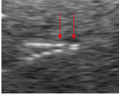
Figure 3.28. Example of lateral resolution visual assessment on an image - targets at 11 cm depth (detail).
