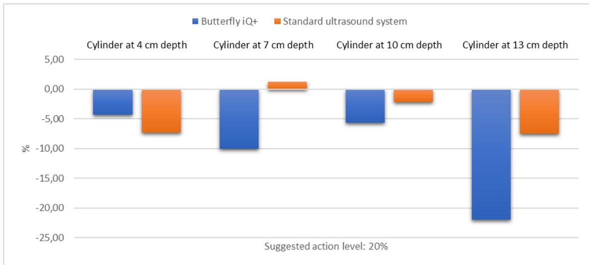
*Figure 3.15. Major geometric distortion in terms of deviations from unitary Aspect Ratio.*
