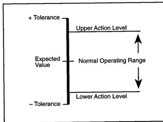
Figure 3.3. Action and defect levels [19].
