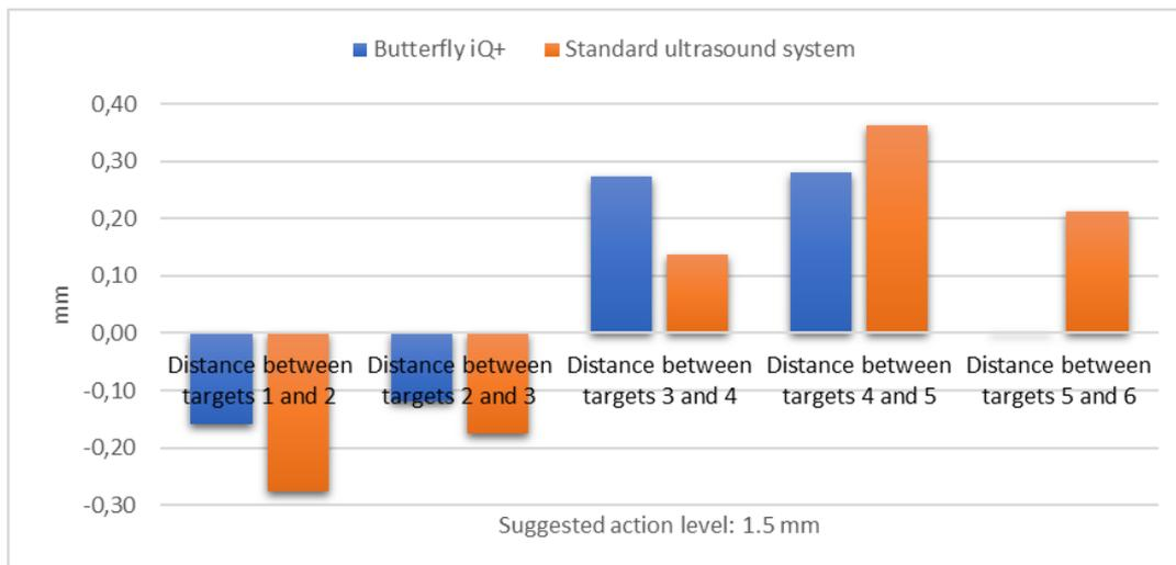
Figure 3.12. Horizontal distance measurement errors.
