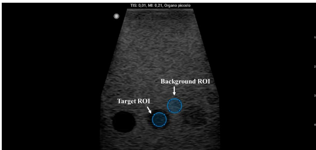
Figure 3.33. Example of selection of ROIs for contrast evaluation of one target with respect to background.
