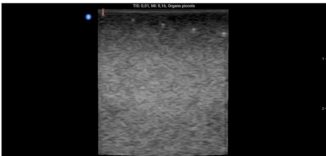
Figure 3.16. Example of dead zone distance measurement on an image.
