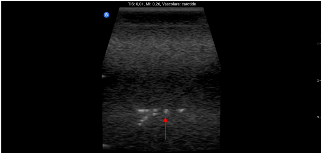
Figure 3.19. Example of axial resolution visual assessment on an image - targets at 3 cm depth.
