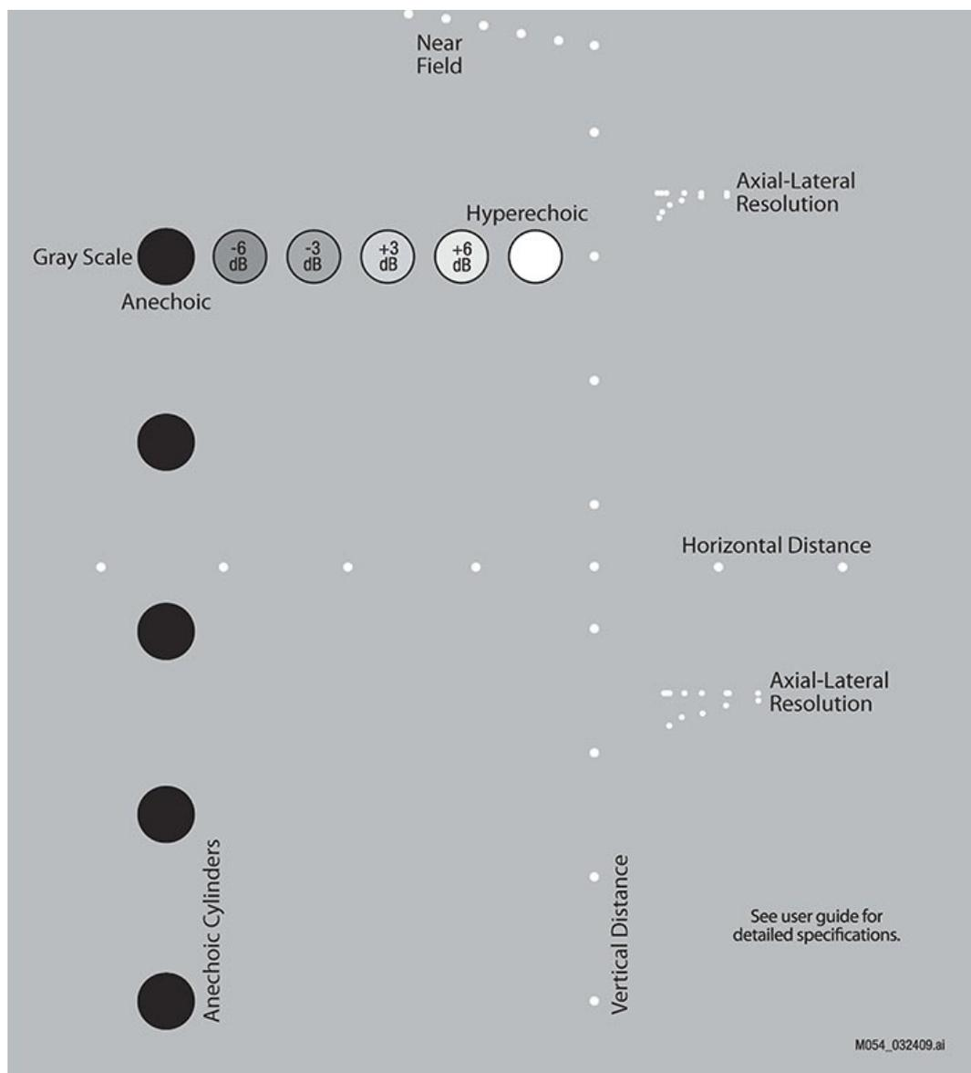
Figure 3.2. Schematic of targets embedded in CIRS phantom - Model 054GS [18].
