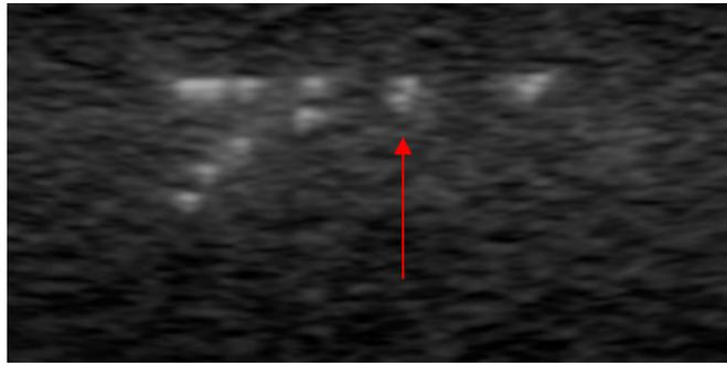
Figure 3.20. Example of axial resolution visual assessment on an image - targets at 3 cm depth (detail).
