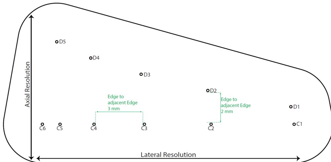
Figure 3.6. Combined Axial/Lateral resolution targets at 11 cm depth [18].
