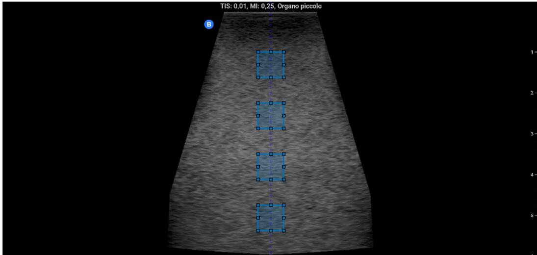
Figure 3.31. Example of automatic ROIs definition for image uniformity assessment.
