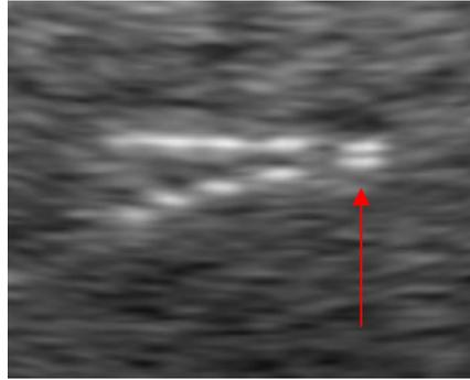
Figure 3.22. Example of axial resolution visual assessment on an image - targets at 11 cm depth (detail).
