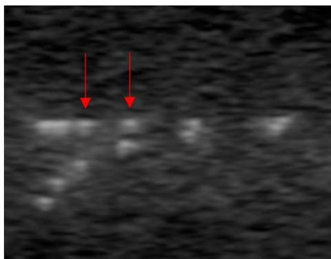
Figure 3.26. Example of lateral resolution visual assessment on an image - targets at 3 cm depth (detail).
