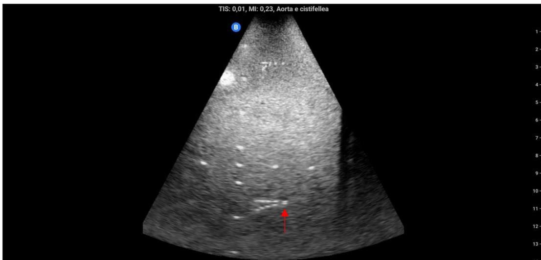
Figure 3.21. Example of axial resolution visual assessment on an image - targets at 11 cm depth.
