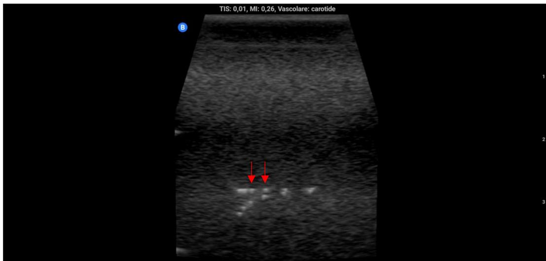
Figure 3.25. Example of lateral resolution visual assessment on an image - targets at 3 cm depth.
