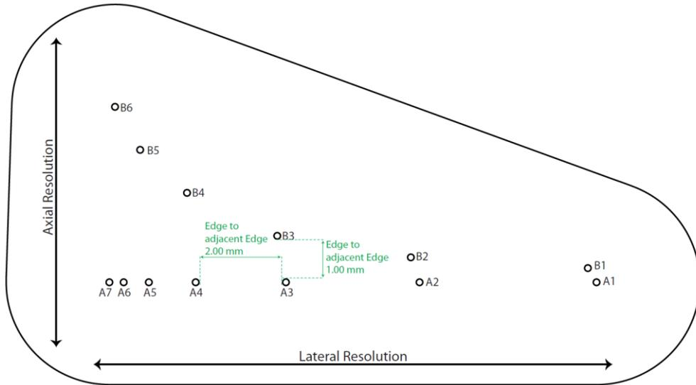
Figure 3.5. Combined Axial/Lateral resolution targets at 3 cm depth [18].
