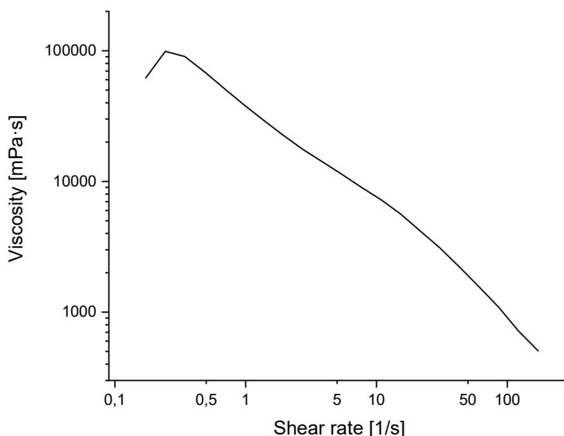
Figure 18. Viscosity versus shear rate for the 5 % (w/v) – 1% hydrogel. Axis in logarithmic scale.
