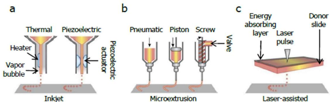
Figure 9. Mainly components of the three 3D bioprinter technologies: inkjet, microextrusion and laser-assisted bioprinter. Reprinted from [47].
