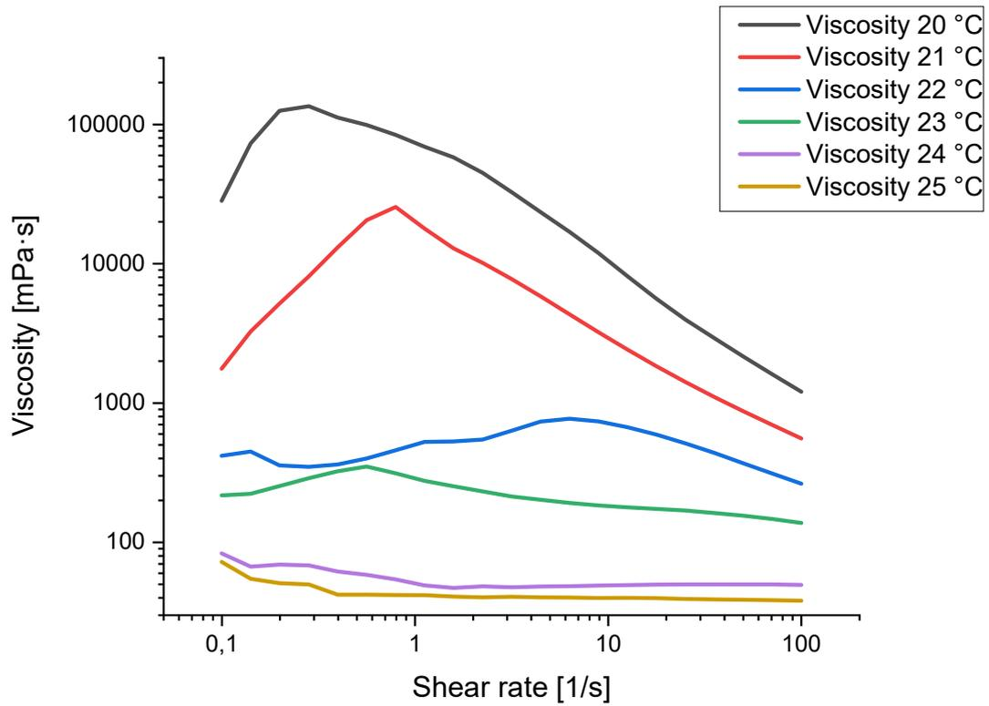
Figure 30. Viscosity versus shear rate for the 5 % (w/v) – 1% hydrogel at different temperatures. Axis in logarithmic
