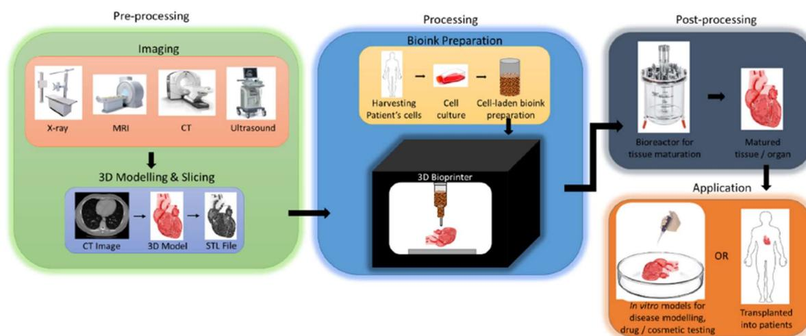
Figure 8. The bioprinting process flow. The pre-processing consists of modelling the construct. The processing consists of effective bioprinting, and post-processing provides the conditions for cell growth. Reprinted from [45].
