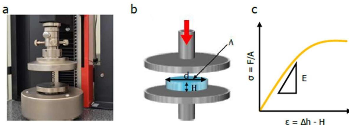
Figure 13. Compression test. A) photograph of the Zwick-Roell Zwicki machine employed. B) Schematic illustration of the compression test and C) representation of stress ( $\sigma$ )-strain ( $\epsilon$ ) curve to compute the Young's modulus. Reprinted from [9].
