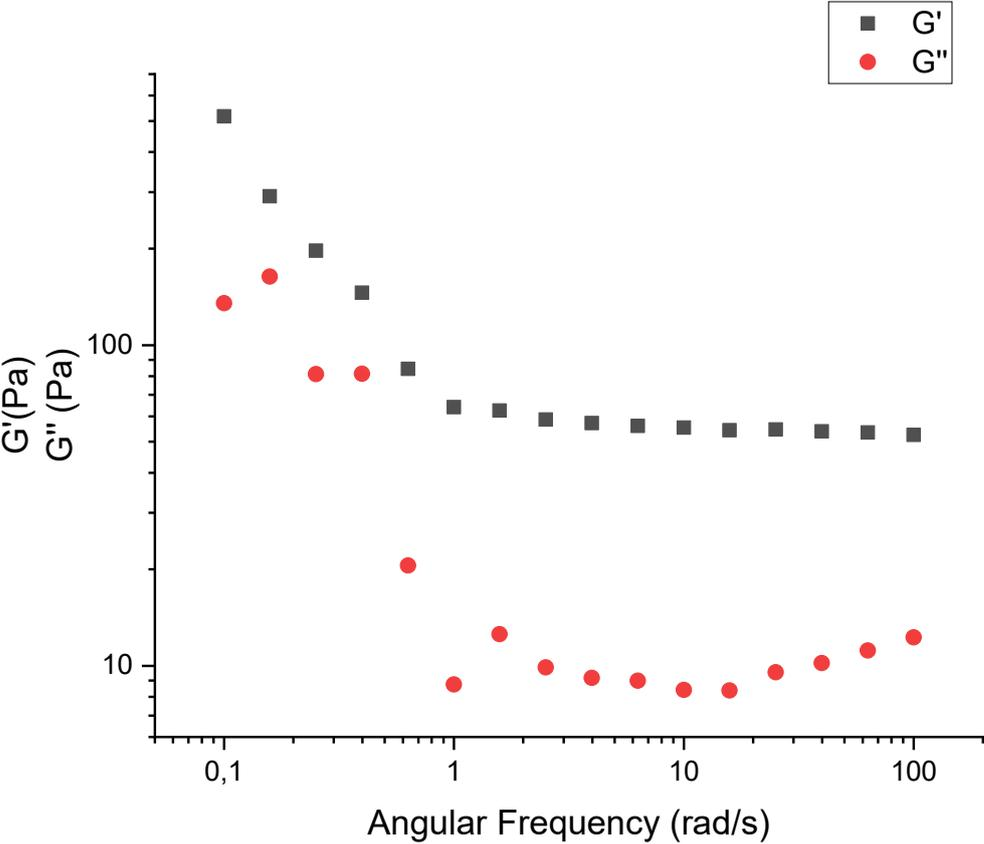
Figure 24. Storage modulus and loss modulus versus angular frequency (oscillatory shear strain = 0.1 %). Axis in logarithmic scale.
