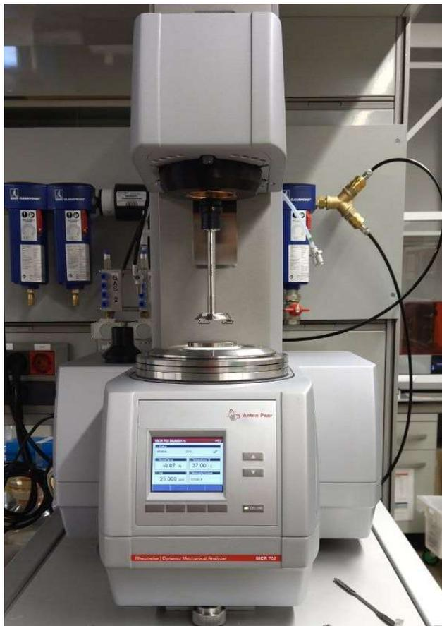
Figure 14. Photograph of the Anton Paar (MCR 702) rheometer.
