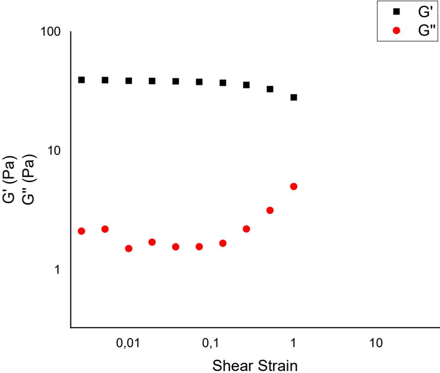
Figure 19 Storage modulus and loss modulus versus oscillatory shear strain (frequency = 1 Hz). Axis in logarithmic scale.
