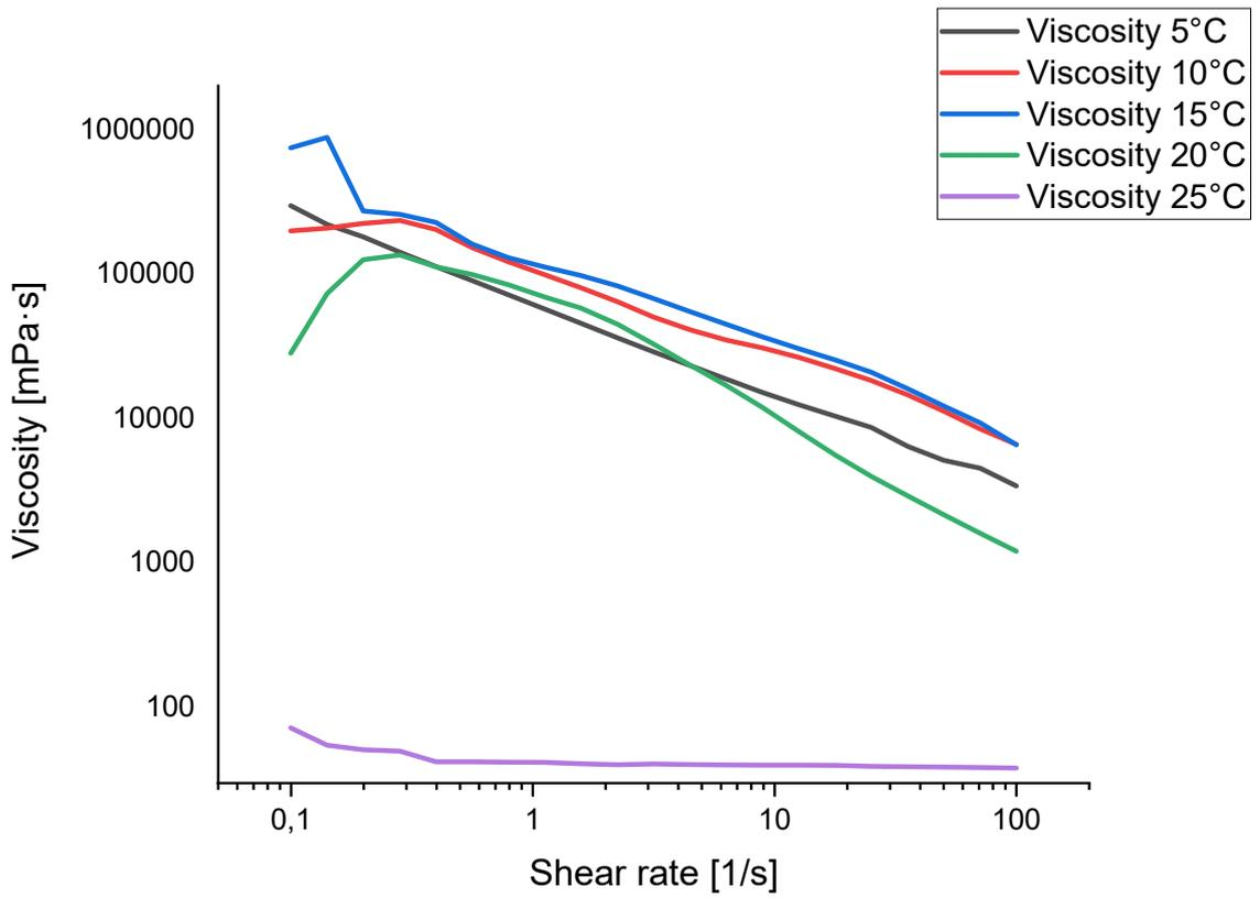
Figure 29. Viscosity versus shear rate for the 5 % (w/v) – 1% hydrogel at different temperatures. Axis in logarithmic scale.
