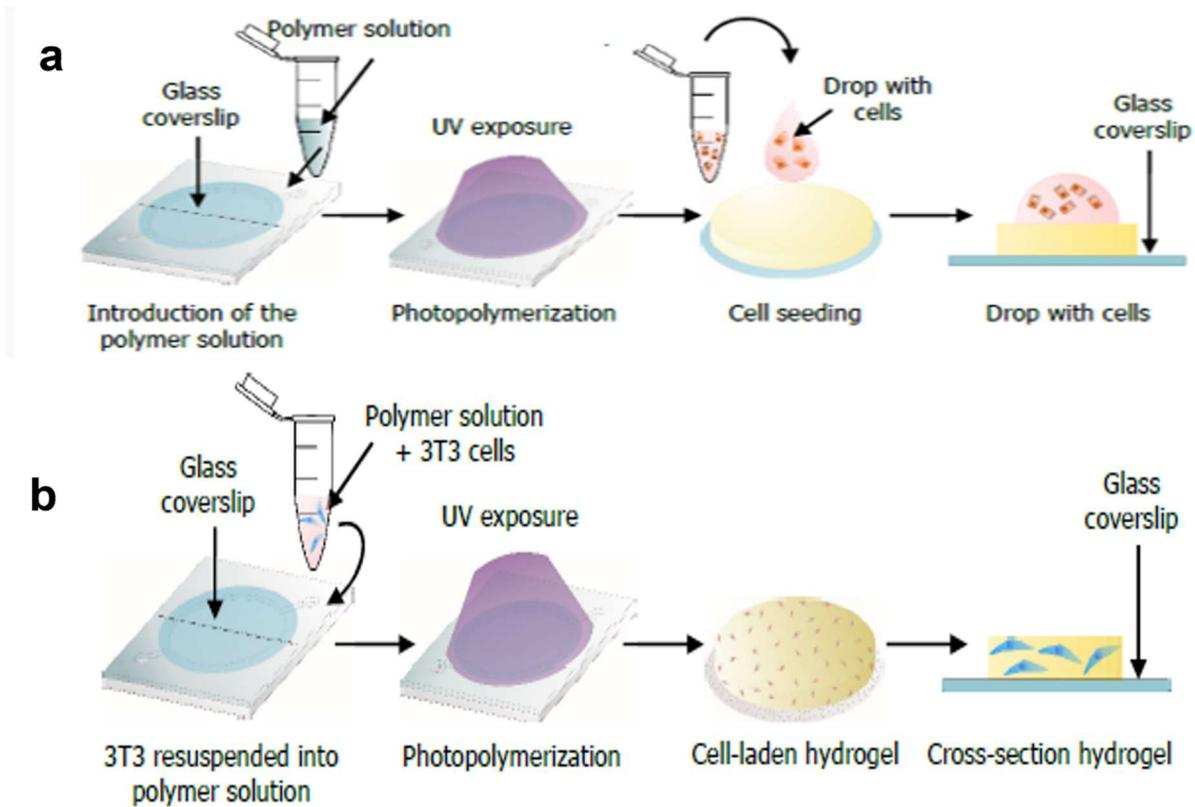
Figure 12. Representation of the hydrogel fabrication process. Polymer solution was poured into PDMS pools covered by a silanized glass slide by a narrow inlet channel and then, photopolymerized. On the top production of hydrogels with a monolayer of cells is shown (a). In the bottom image, cell-laden hydrogel fabrication is represented (b). Reprinted from [9].
