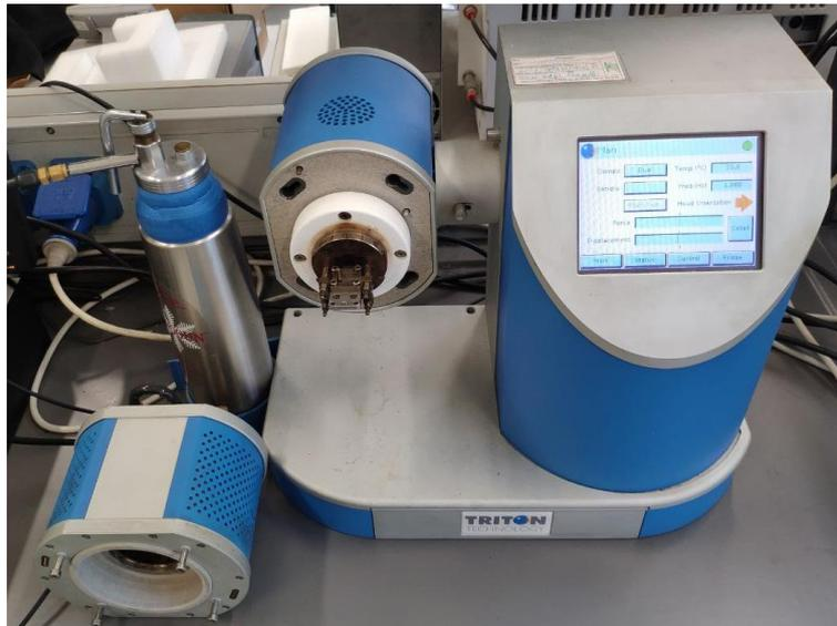
Figura 3.11: TTDMA Triton Technology-Mettler Toledo
