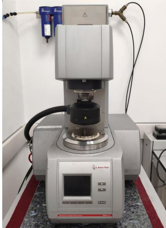
Figura 3.6: Reometro Anton Paar MCR 302
