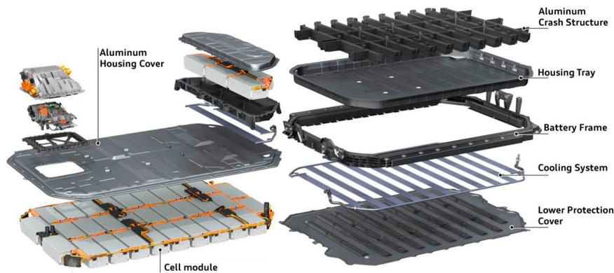
**Figure 3.8:** Audi e-tron battery pack [81]
