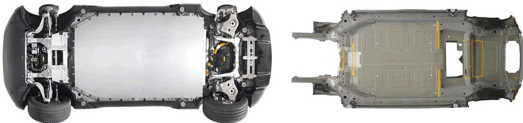
**Figure 1.8:** Jaguar I-pace underbody-battery pack integration, underside view [10]
