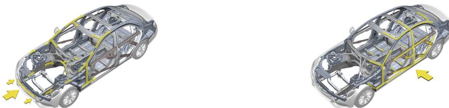
**Figure 2.3:** Mercedes Benz C-class front and side impact schematic load path [43]
