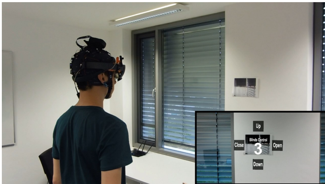
Figure 13: Window Blinds control via AR using the SSVEP-BCI paradigm in a room ( Putze et al., 2019 ).
