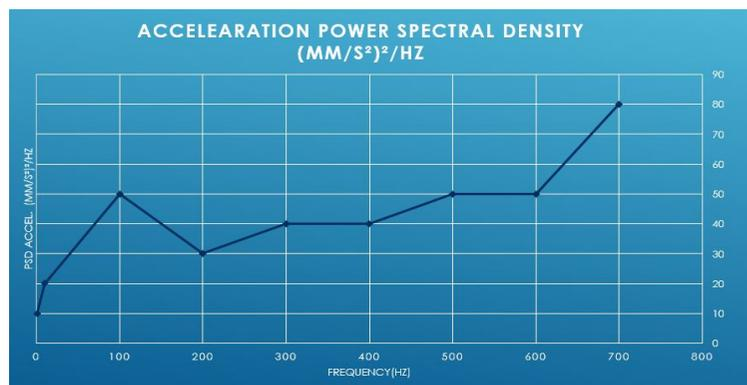
Figure 5.20: Power Spectral Density of the Acceleration applied in the -Y direction on the solar panel surface
