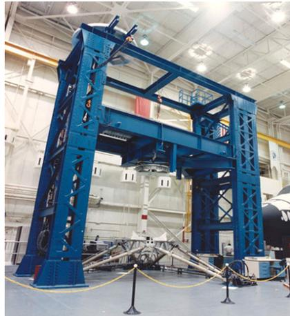
**Figure 1.2:** Six Degrees of Freedom Dynamic Test System in the Johnson Space Center in USA
