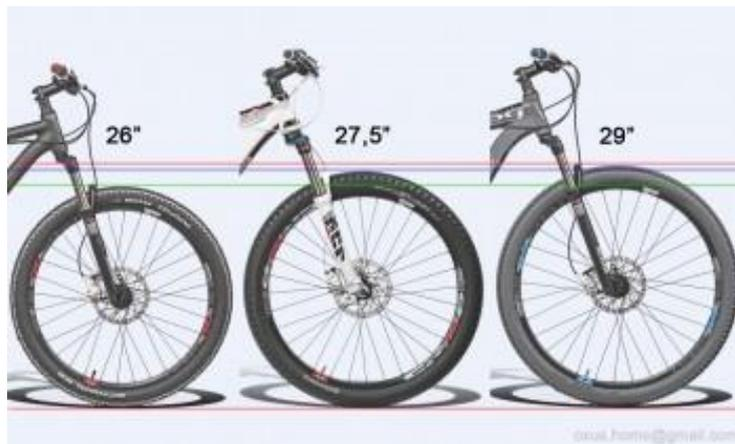
Figura 2.7 Differenti diametri ruota, "<https://mtbpiemonte.com/mtb-dimensione-diametro-ruote-275-o-29-differenza-e-confronto/>"
