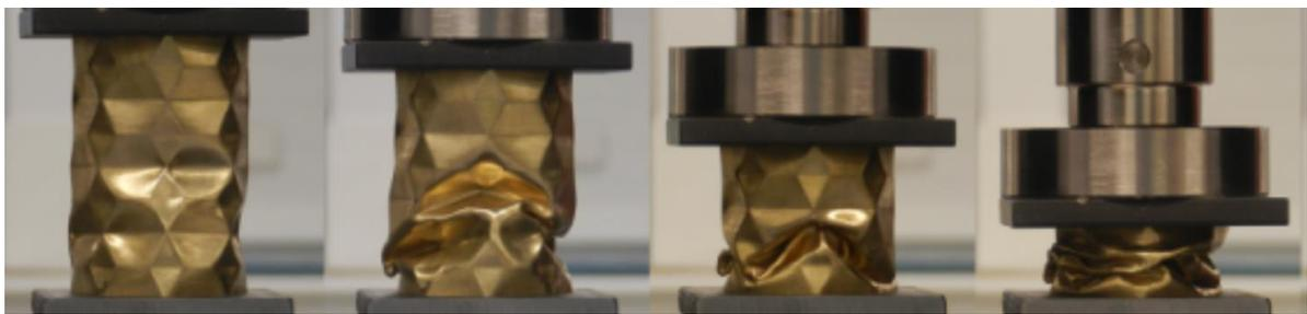
*Figure 20 Crushing of origami patterned 3D printed brass tube [39]*
