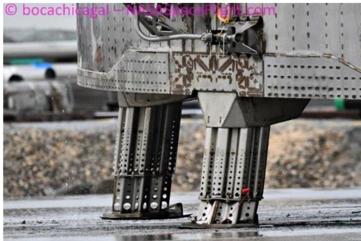
*Figure 5 SpaceX Starship SN6 energy absorbers [20]*
