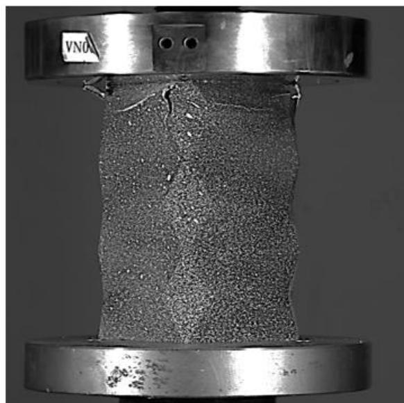
*Figure 55 AlSi10Mg specimen fractures*
