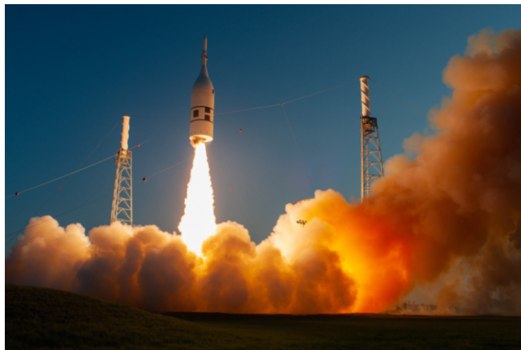
Figure 4.17. A launch abort system with a test version of Orion attached soars upward on NASA's Ascent Abort-2 (AA-2) flight test atop a Northrop Grumman provided booster on July 2, 2019. Credits: [21].
