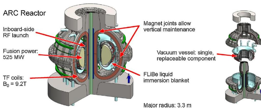
Figure 1 design and dimension of ARC. [3]
