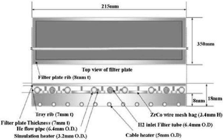
Figure 11 Cross section and top views of a tray. [15]
