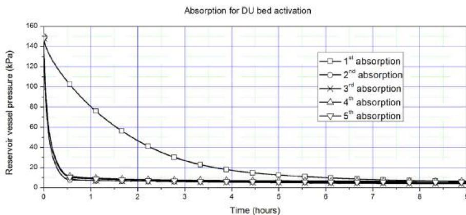
Figure 9 Absorption of hydrogen during DU bed activation – Pressure changes in vessel. [15]
