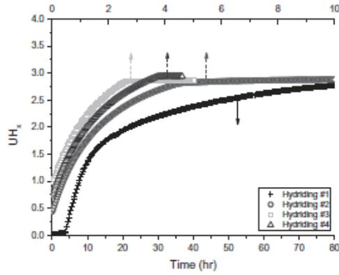
Figure 8 The ratio of hydrogen absorption in the storage material over time. [14]
