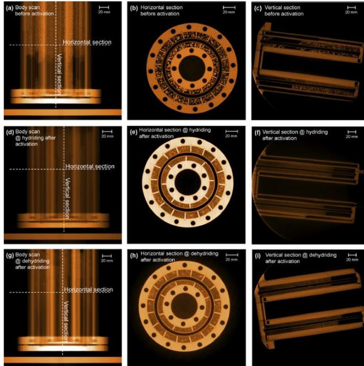
Figure 15 ICT images of the ZrCo bed before activation (a–c), after activation at state of hydriding (d–f), after activation at state of dehydriding (g–i). (a), (d), (g): scan of the bed body; (b), (e), (h): horizontal section; (c), (f), (i): vertical section. [15]
