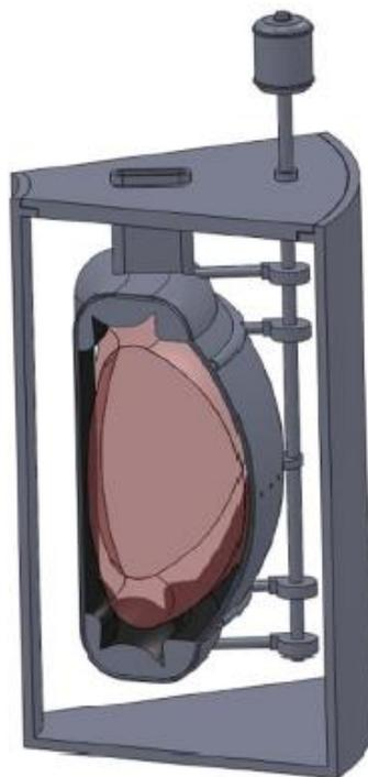
Figure 2 Double-walled vacuum vessel design with FLiBe coolant channel. [3]
