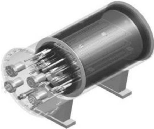
Figure 10 3D model of the ZrCo bed. [15]
