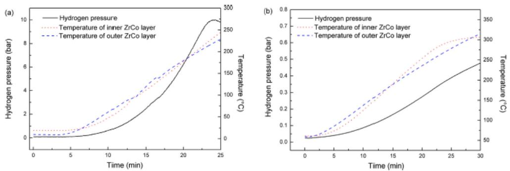
Figure 14 Evolutions of hydrogen pressure inside the ZrCo bed before hydrogen delivery when heating the bed under mode 1 (a) and mode 2 (b). [15]
