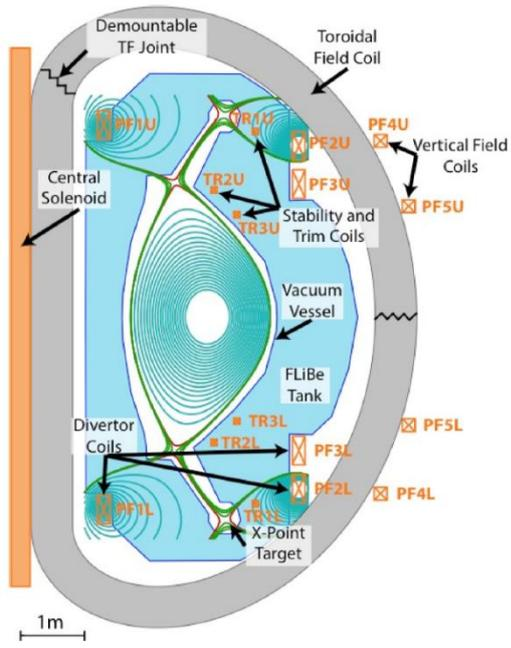
Figure 3 Magnetic equilibrium, coils set, vacuum vessel and FLiBe tank geometry of ARC. [4]
