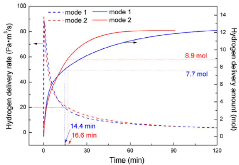
Figure 13 Hydrogen delivery amount curves and average hydrogen delivery rate curves of the ZrCo bed under delivery mode 1 and mode 2 at 400 °C. [12]
