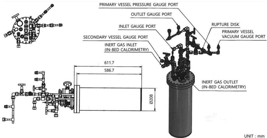
Figure 6 Outer shape of a DU bed. [12]
