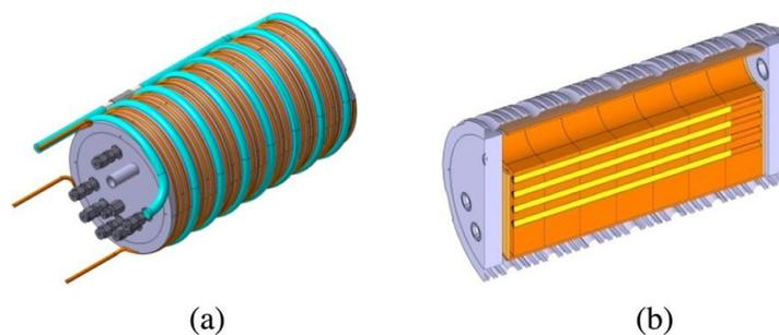
Figure 7 Major design features of current DU bed (a) Primary vessel brazed with electrical heaters and cooling channels (b) DU rods (yellow) loaded into holes in copper foam (orange). [13]
