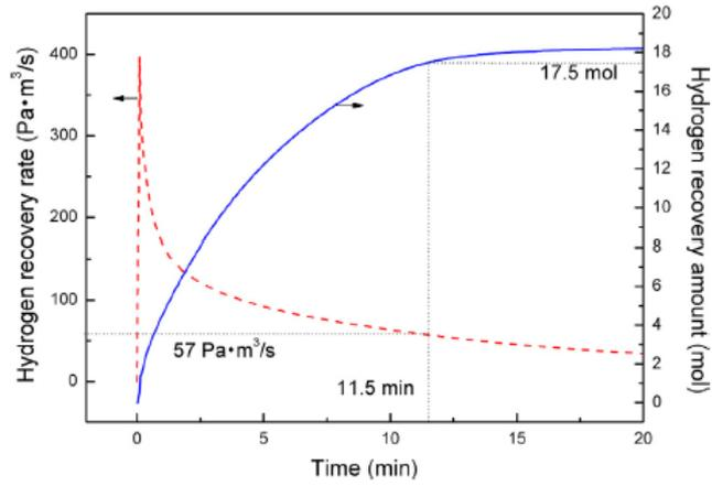
Figure 12 Hydrogen recovery amount curve and average hydrogen recovery rate curve of the ZrCo bed. [12]
