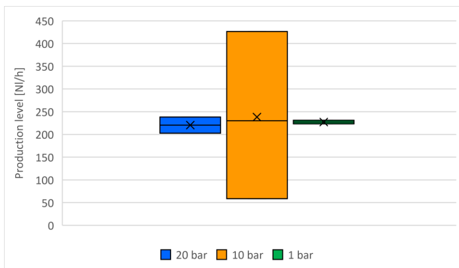
Figure 10 - Representation of the mean production level and its standard deviation for different hydrogen outlet pressures, when the setpoint production is equal to 300 l/h
