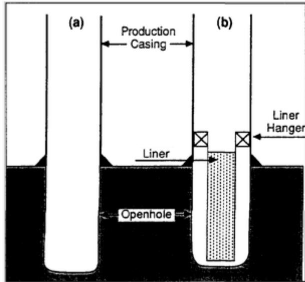
Figure 23 – Open hole completion (a) and liner completion (b)
