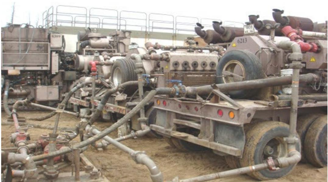
Figure 12 – Pumping units for hydraulic fracturing
