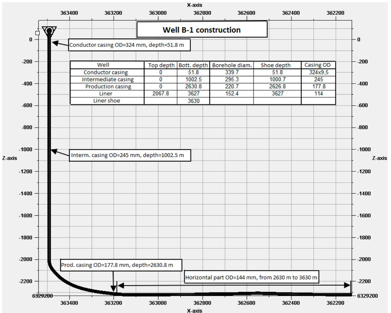
Figure 19 – Well B-1 construction
