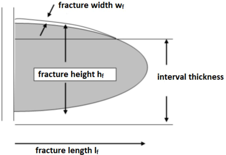
Figure 5 – Fracture geometry
