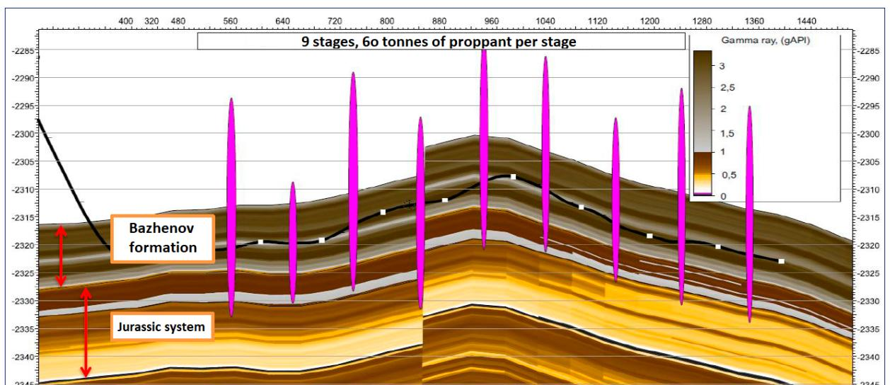
Figure 21 – Geologic cross-section and hydraulic fracturing stages
