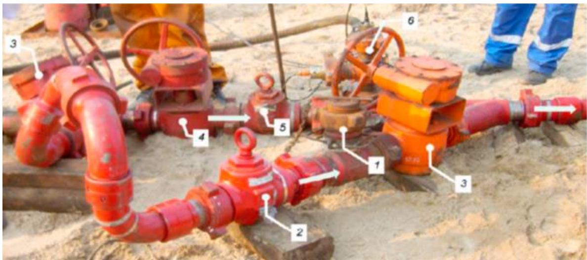
Figure 18 – Auxiliary line for launching balls into the well
