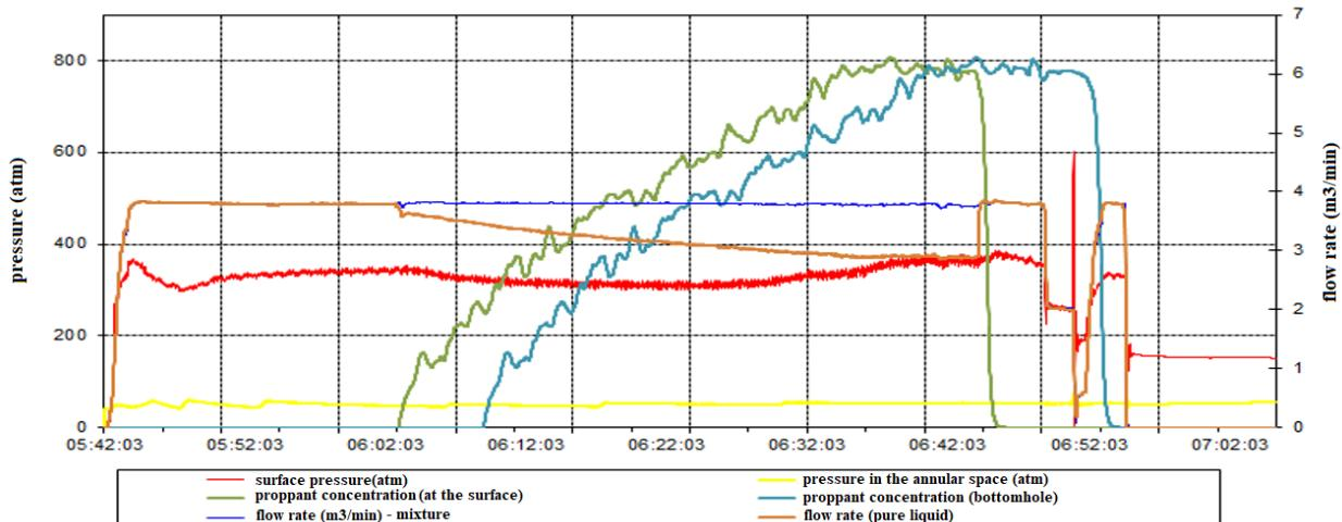
Figure 24 – Graph of Multistage Hydraulic fracturing (stage 2)
