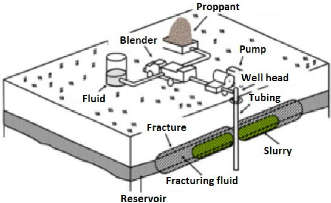
Figure 6 – Hydraulic fracturing scheme
