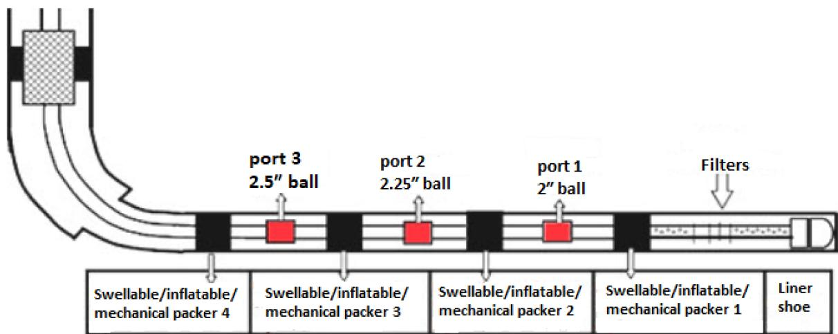
Figure 15 – General completion scheme for multistage hydraulic fracturing
