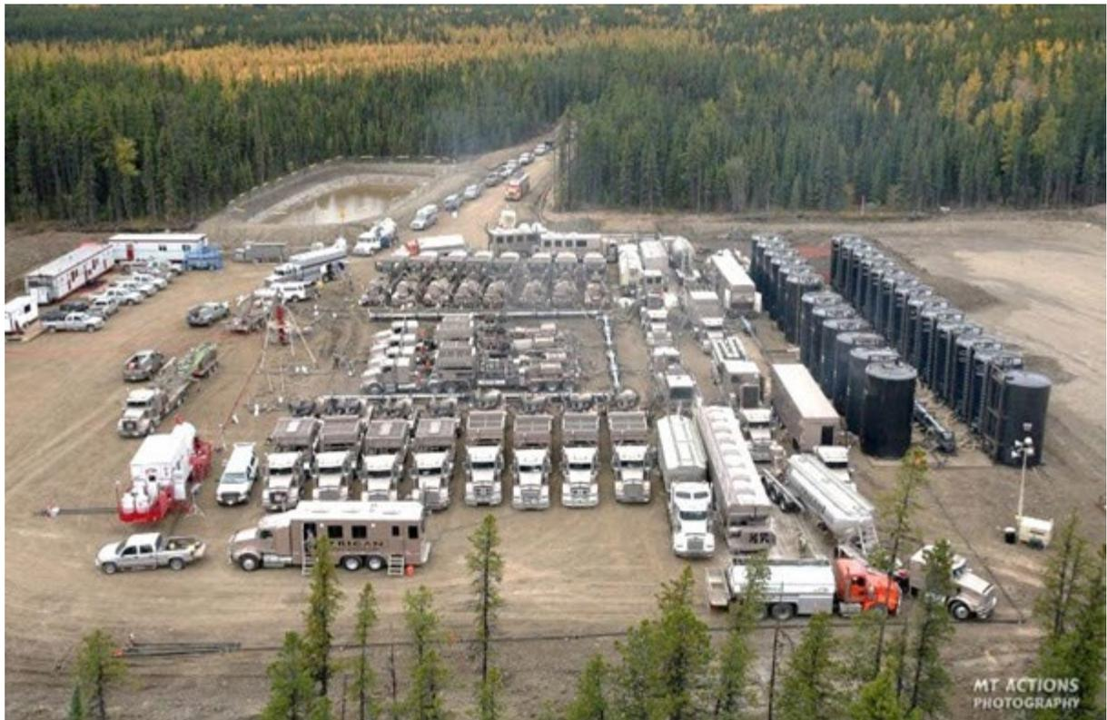
Figure 13 – General layout of equipment for large-volume hydraulic fracturing
