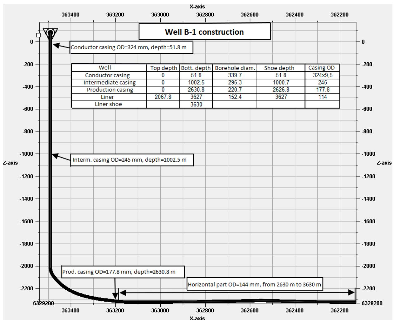
Figure 19 – Well B-1 construction
