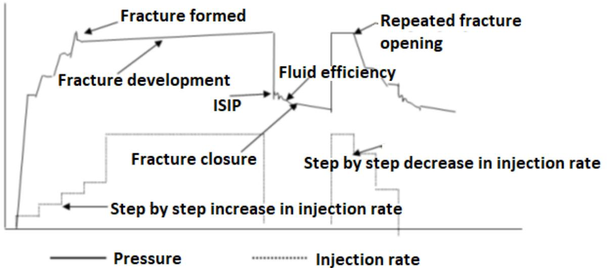
Figure 8 – Bottomhole pressure record during Mini-frac Test
