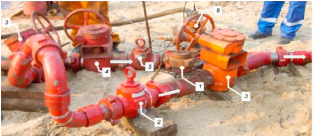
Figure 18 – Auxiliary line for launching balls into the well
