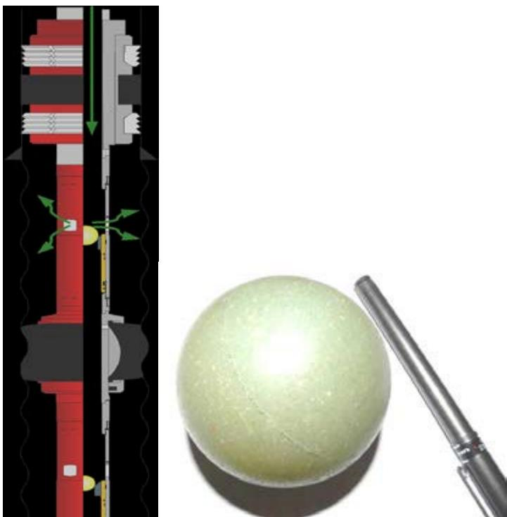
Figure 16 – Single-action system with frac sleeve activated by ball drop
