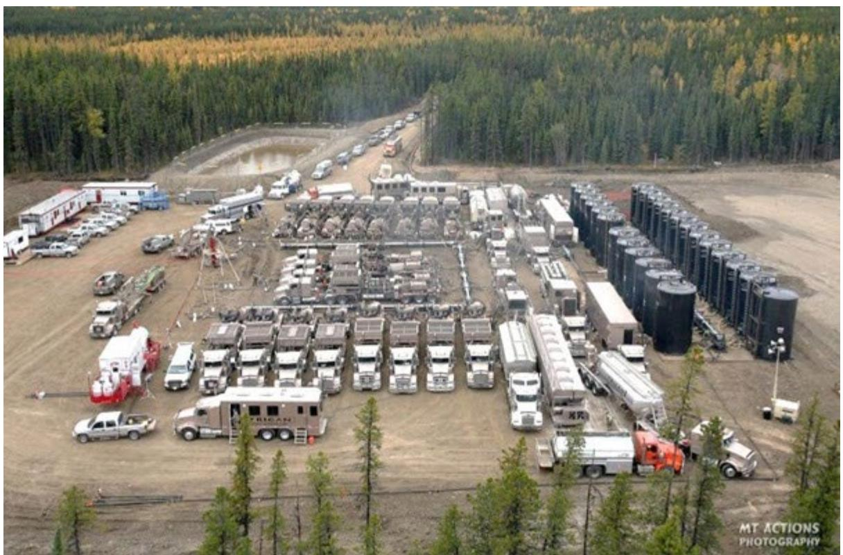
Figure 13 – General layout of equipment for large-volume hydraulic fracturing
