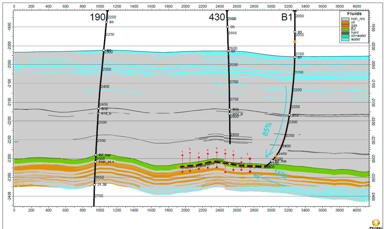
Figure 22 – Geologic cross-section with possible directions of water breakthrough
