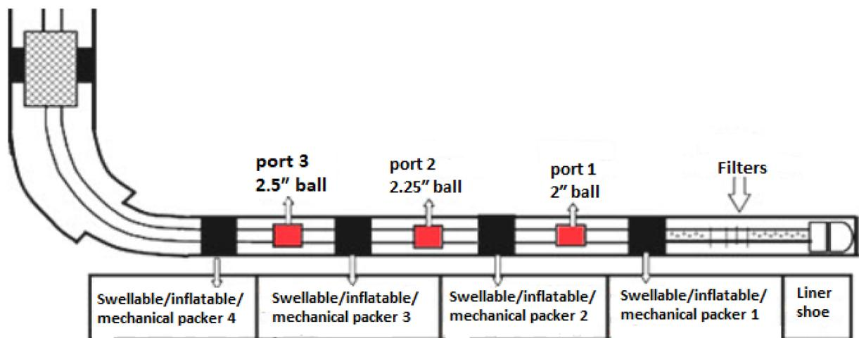
Figure 15 – General completion scheme for multistage hydraulic fracturing
