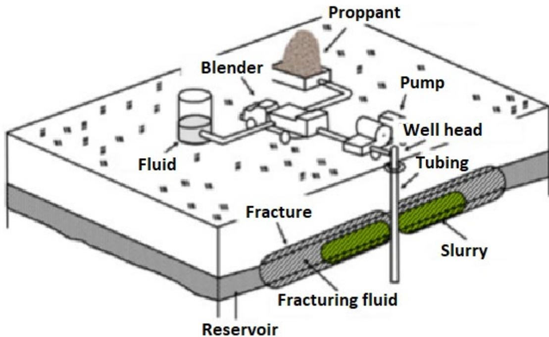
Figure 6 – Hydraulic fracturing scheme
