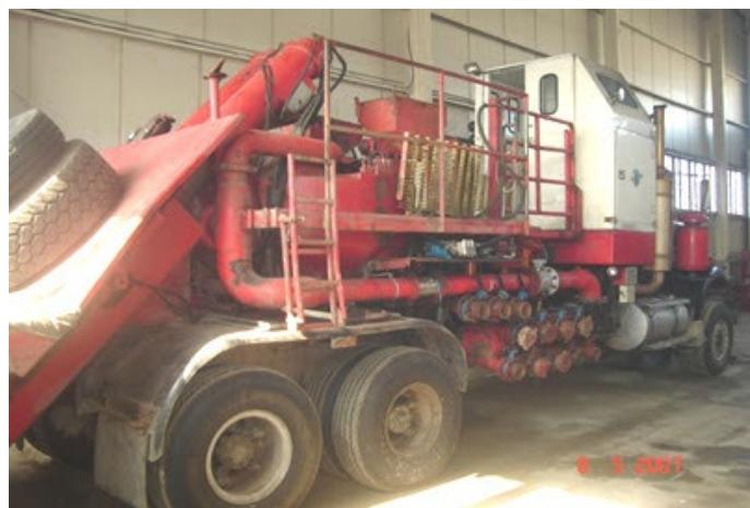
Figure 11 – Example of a mixing unit (blender)
