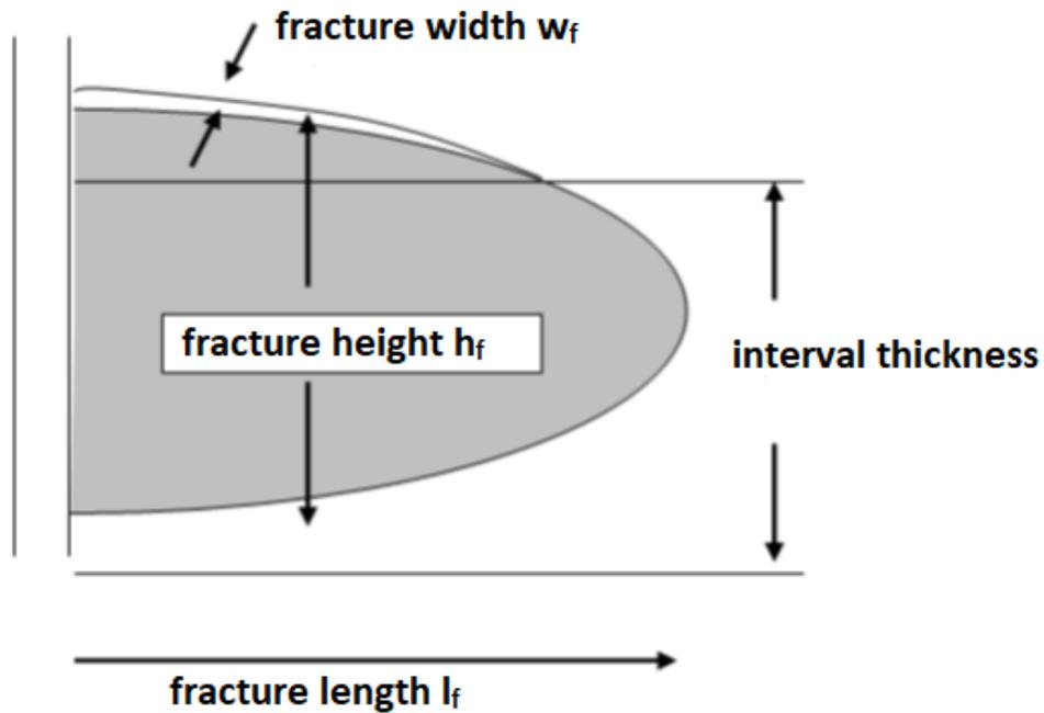
Figure 5 – Fracture geometry
