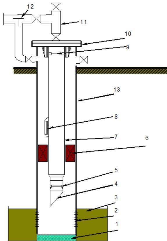
Figure 10 – Subsurface equipment for hydraulic fracturing:
