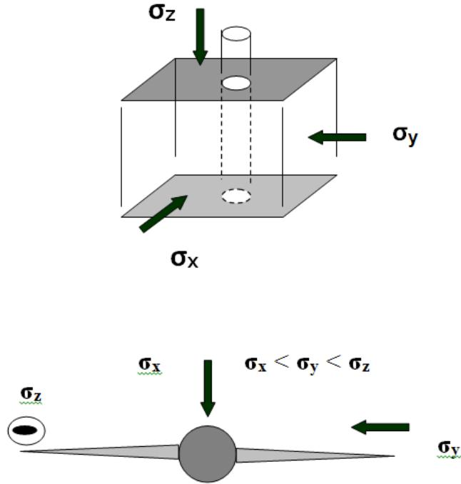
Figure 7 – Image of a vertical fracture perpendicular to  $\sigma_x$
