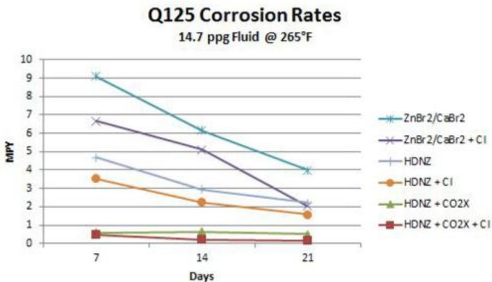
Figure 9. General corrosion rates depending on different brines
