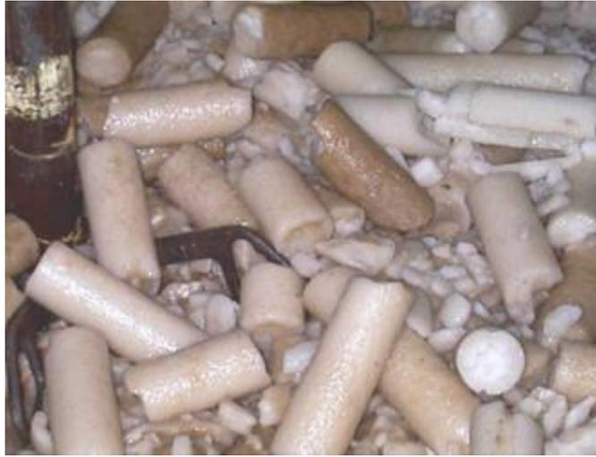
Figure 4. Precipitated salt crystals
