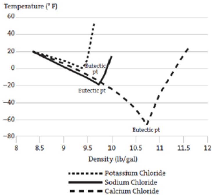
Figure 6. Crystallization temperature curves for KCl, NaCl, CaCl<sub>2</sub>
