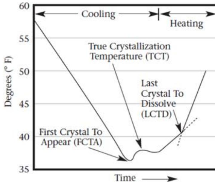
Figure 3. Different points of crystallization
