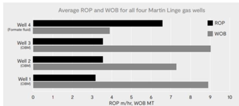
Figure 8. ROP increased significantly despite the low WOB due to application of cesium/potassium formate.
