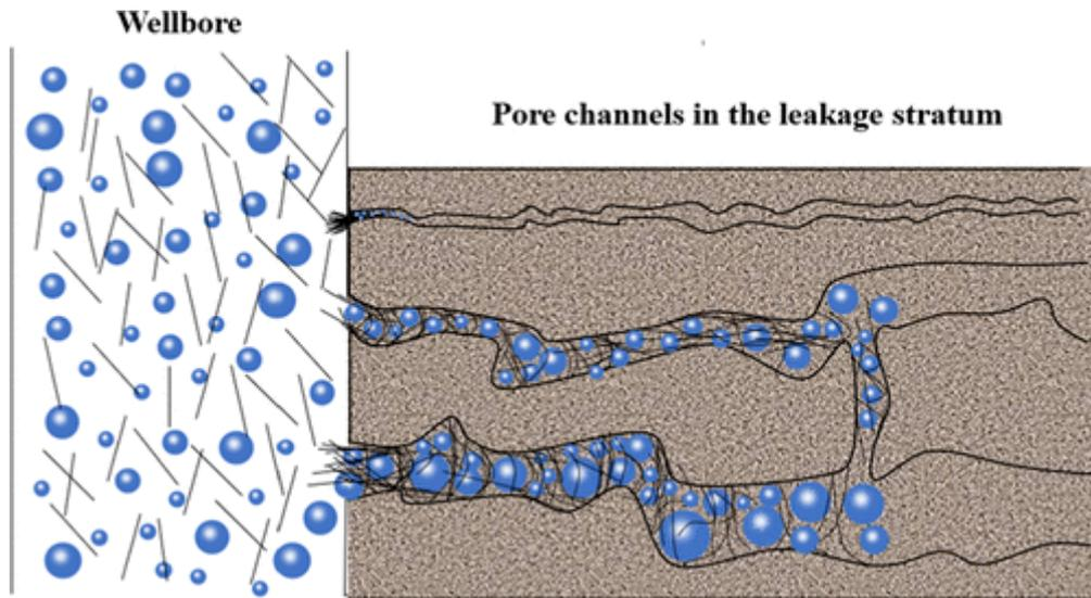
Figure 12. Plugging mechanism formed by solid particles and fiber in the pore channel of leakage formation.
