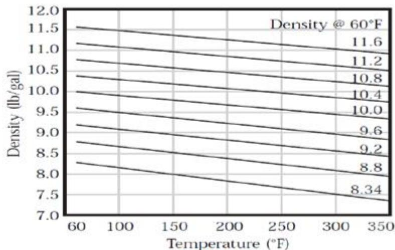
Figure 1. CaCl<sub>2</sub> density reduction in case of thermal expansion.
