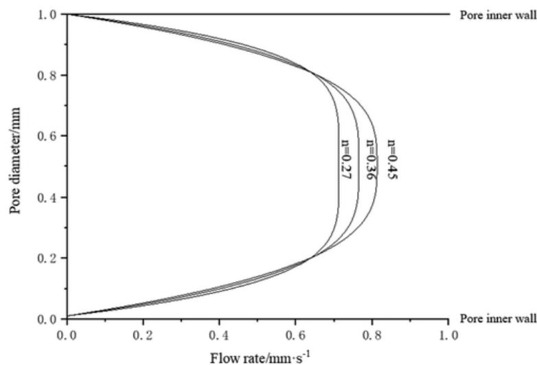
Figure 14. Effect of fiber concentration on the flow behavior of four kinds of fiber suspensions in pore space.
