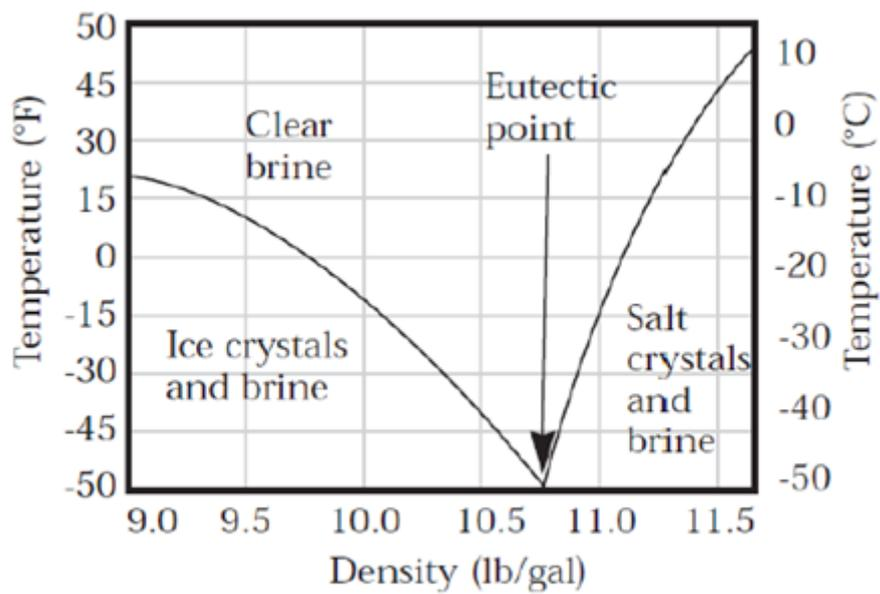
Figure 2. Density effect of CaCl<sub>2</sub> brine on the crystallization temperature.
