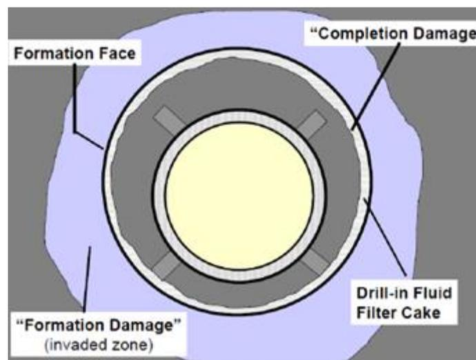
Figure 7. Well damage types
