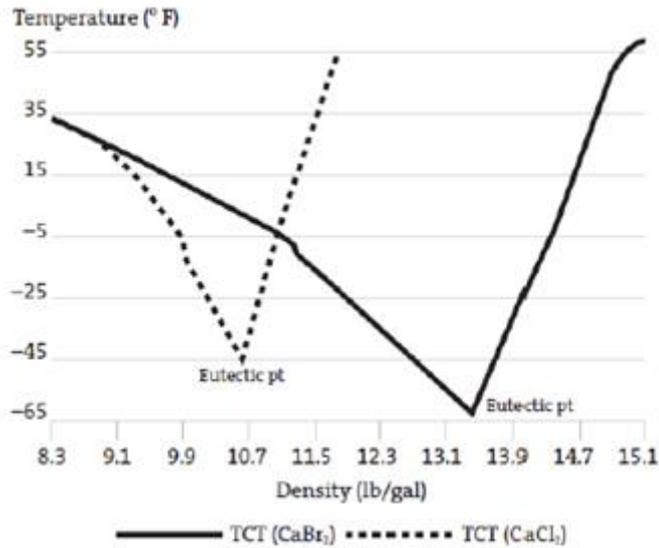
Figure 5. Crystallization temperature curves for CaBr<sub>2</sub> and CaCl<sub>2</sub>
