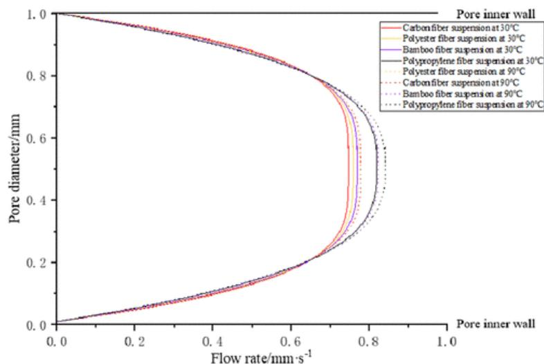
Figure 15. Flow behavior of different fiber suspensions in pores at 30 and 90°C.
