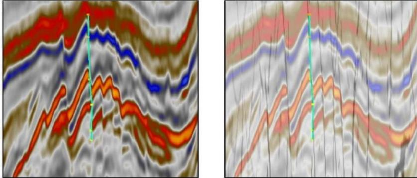
*Figure 3.1: Manual fault interpretation (light blue) from post-stack amplitude (Haibin Di, et al., 2017)*
