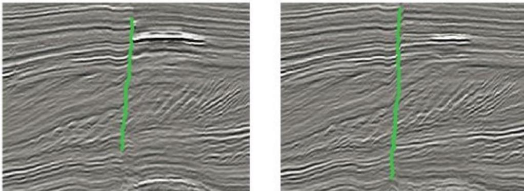
*Figure 3.2: Semi-automatic fault extraction as shown in two seismic sections (Zhen Wang, Long, et al., 2014)*
