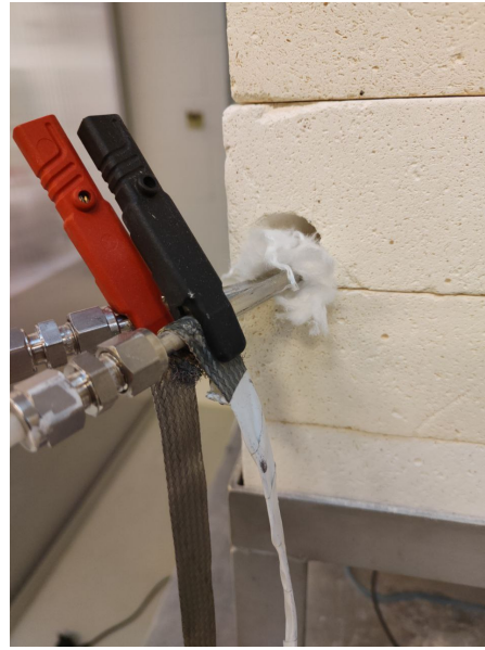
(b) Wires stapled to the outlet pipes
