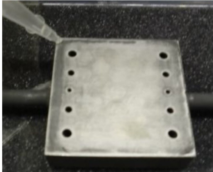
Figure 4.4: Superglue application on the fuel-electrode [35]
