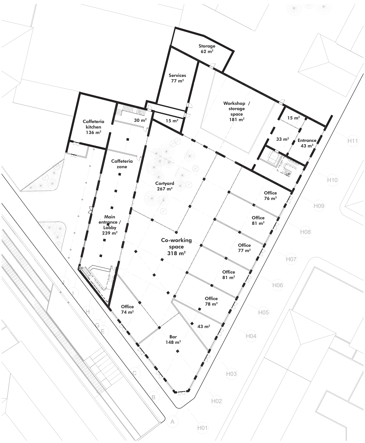
GROUND FLOOR PLAN
