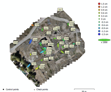
Fig. 4. GCP locations and error estimates. Z error is represented by ellipse color. X,Y errors are represented by ellipse shape. Estimated GCP locations are marked with a dot or crossing.
