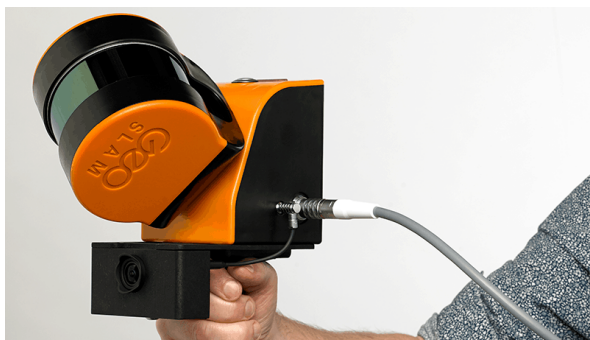
Fig. 3.30: Laser scanner mobile ZEB GO
