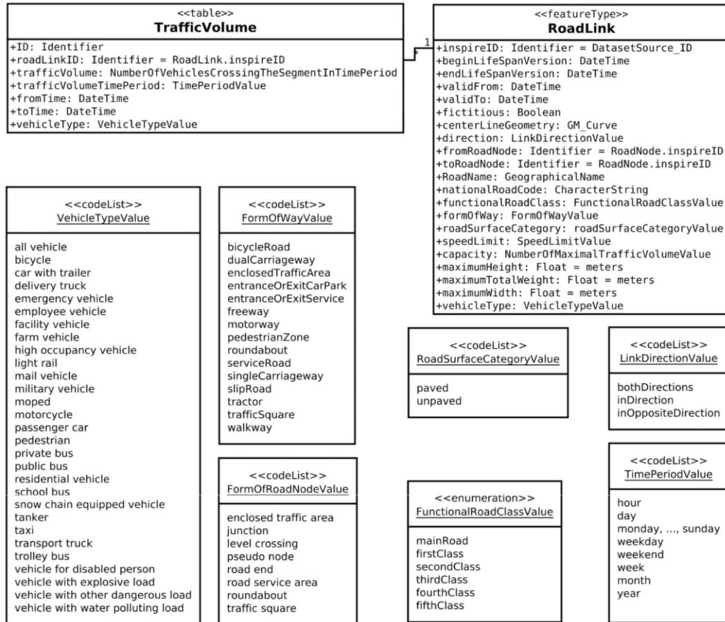
Figure 55. Data model of OTM is based on OpenStreetMap attributes and code lists. Data structure is filled with information that respect OSM data values. [source:
