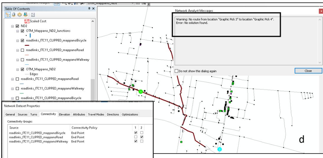
Fig. 76c. Directions and routes are generated when all roads are in the same level of connectivity, hence interacting with each other [source: author]
