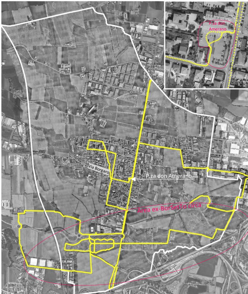
Figure 70. Mapped points through RTK GNSS system extraction resulted as an apparently single line since points were collected every two seconds. Yellow is for the points [source:author]
