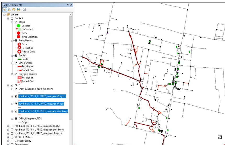
Figure 76a, 76b, 76c, 76d. Network Analysis of the cycling roads show the impossibility for cyclist to reach a destination along the main road (Strada Cuornè) remaining on a cycle path.
