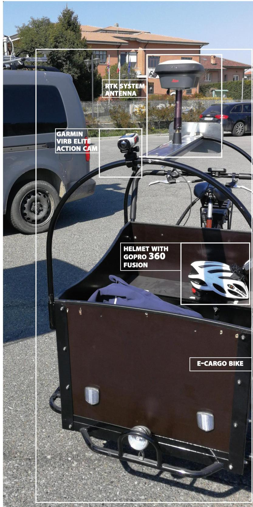
Figure 69. E-cargo bike with mounted equipment used to carry out the recording of spatial data of the municipality of Mappano. [source: author]
