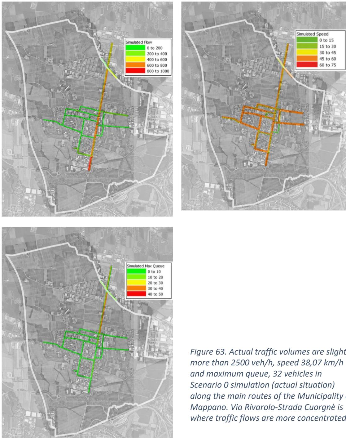
*Figure 63. Actual traffic volumes are slightly more than 2500 veh/h, speed 38,07 km/h and maximum queue, 32 vehicles in Scenario 0 simulation (actual situation) along the main routes of the Municipality of Mappano. Via Rivarolo-Strada Cuornè is where traffic flows are more concentrated.*
