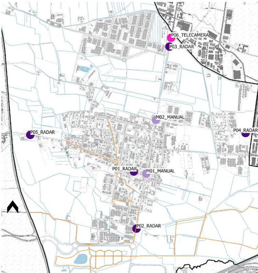
Figure 61. Localization of the 5 radar stations, the camera, the manual surveys superimposed on the cycle paths [source: Traffic Lab data and author]
