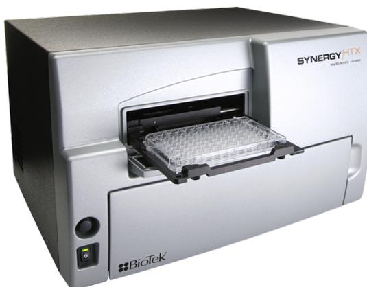
**Figure 3.3.** Synergy HTX Multi-Mode Reader.
