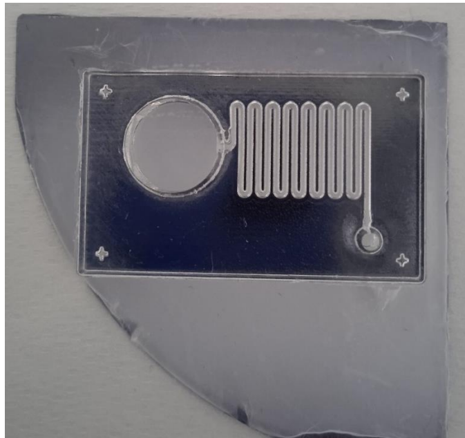
Figure 5.7 - Assembled microfluidic system: the chip has been bonded by interlayer bonding technique, ensuring a good alignment of the channels with respect to the patterned nanofibers
