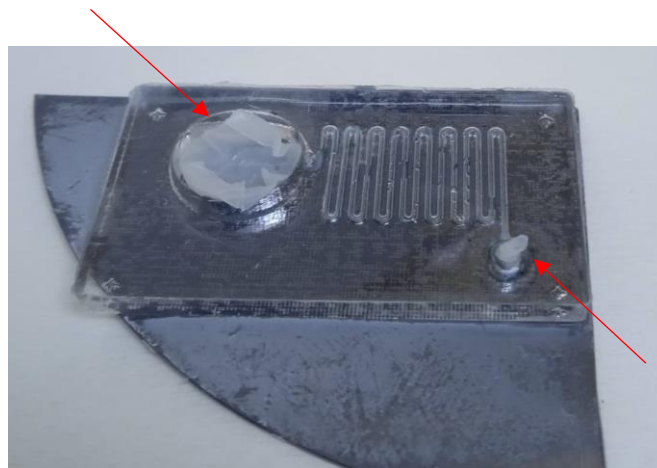
Figure 5.9 - Device subjected to the ethanol leak test; those indicated with red arrows represent the inlet and outlet areas closed with parafilm.
