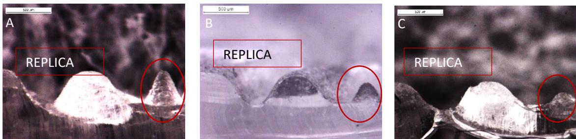
Figure 4.5. Section of A) d200/v75, B) d100/v75, C) d100/v100 samples, scale bar:500  $\mu\text{m}$ . Pillars are circled in red.
