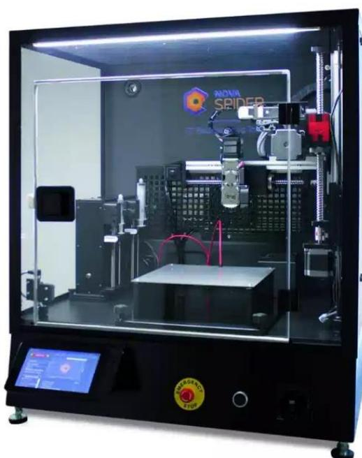
Figure 3.14. Novaspider V5 device.
