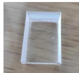
**Figure 4.13.** Photo of the box of alignment produced by laser ablation.
