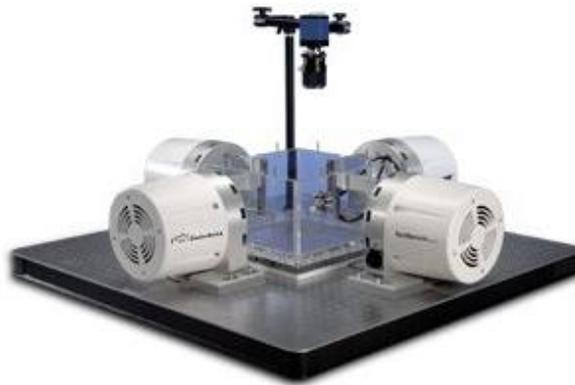
Figure 3.17. Planar biaxial testbench instruments.
