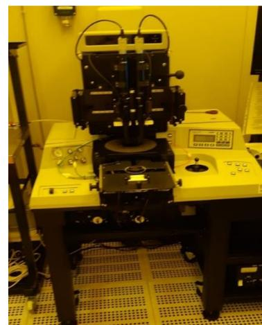
Figure 3.2.5 Workbench: Spin coater – Hot plate- SU-8 2150 - UV photolithography system
