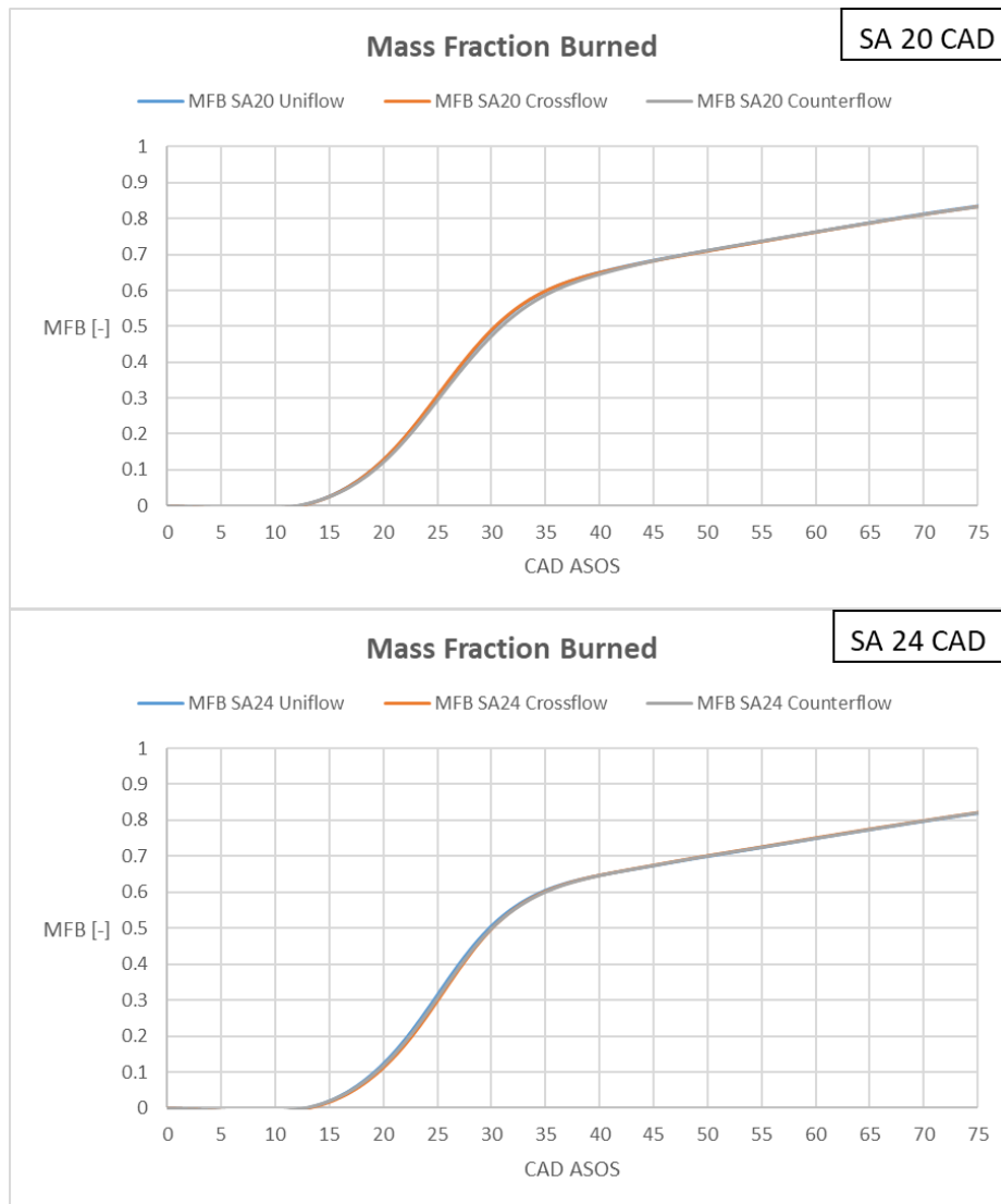
Figure 5. 16, Mass Fraction Burned for \lambda=1.15 and Spark Advance from 8 to 24 CAD.
