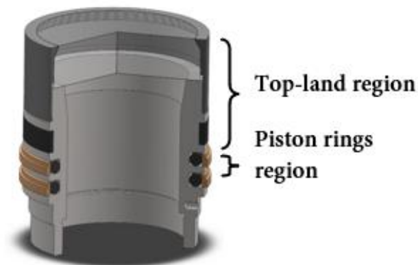
Figure 2. 8, 3D render visualization of piston crown.
