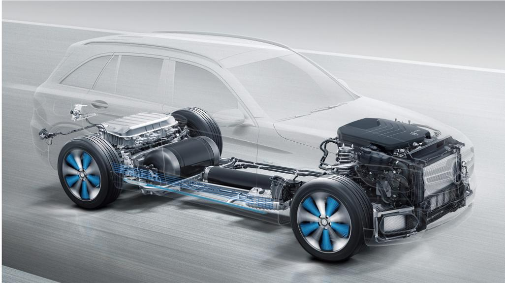
Figure 12 - Mercedes GLC Fuel Cell Powertrain Architecture
