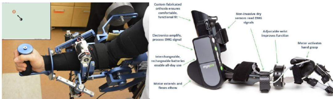
Figure 2.10 MAHI Exo-II rehabilitation exoskeleton [80] (left), MyoPro orthosis [80] (right)
