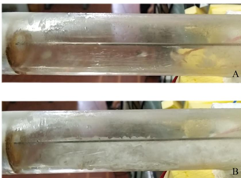
Figure 8.6. **A**: experimental expansion chamber filled with liquid  $N_2O$  at ambient pressure and saturation temperature. **B**:the liquid start to freeze for the effect of a sudden reduction of pressure due to the connection of a vacuum pump.
