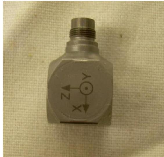
Figure 2.2 - a) The triaxial IEPE accelerometer
