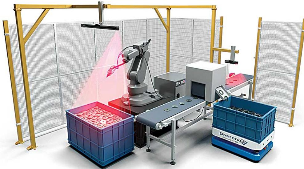
Figure 10: Bin Picking application example [14]
