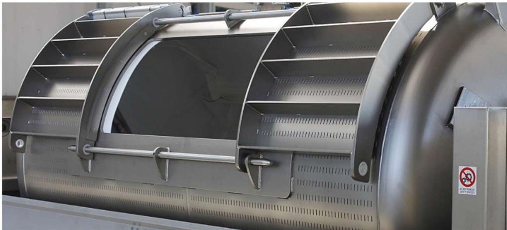
Figure 2.1 Tank forato Pressa F22
