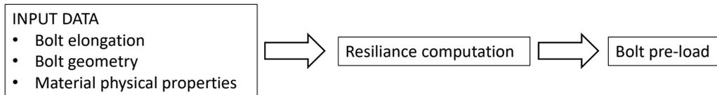
Figure 3.8: Pre-load algorithm calculation scheme
