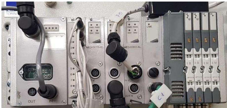
Figura 3.9 CX06 e moduli I/O [14]
