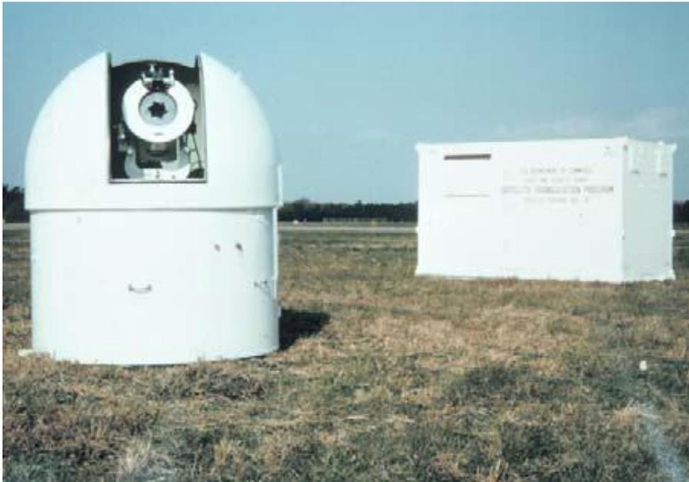
*Figure 21. BC4 Satellite Triangulation Camera station operated by the U.S. Coast and Geodetic Survey. Source: History of Photogrammetry.*
