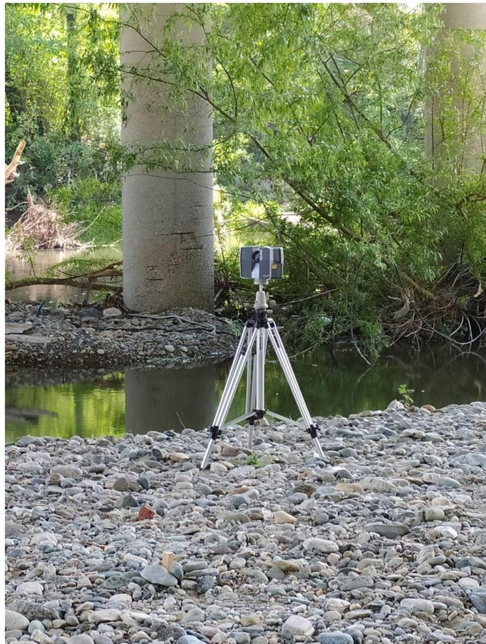
*Figure 106. laser scanner used for the survey of the Stura bridge*
