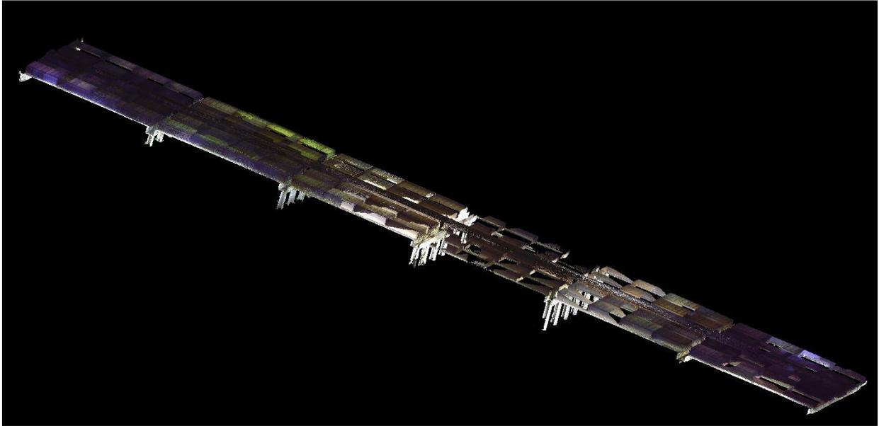
*Figure 138. Dense cloud from laser scanner cleaned*
