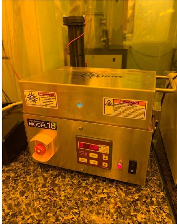
Figure 21: Jetlight UVO-Cleaner® model 18.
