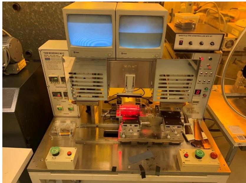
Figure 29: Thermal press.
