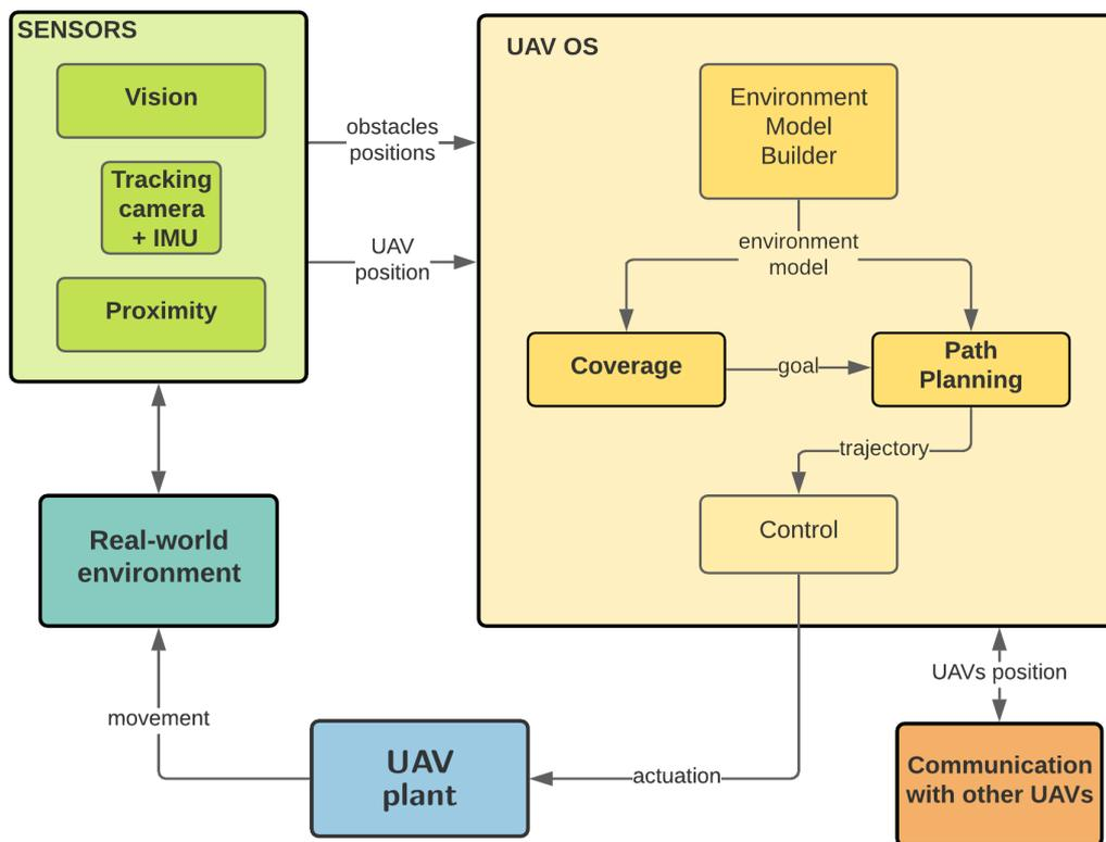
**Figure 4.2:** Block scheme of the simulation environment at an high-level structure.
