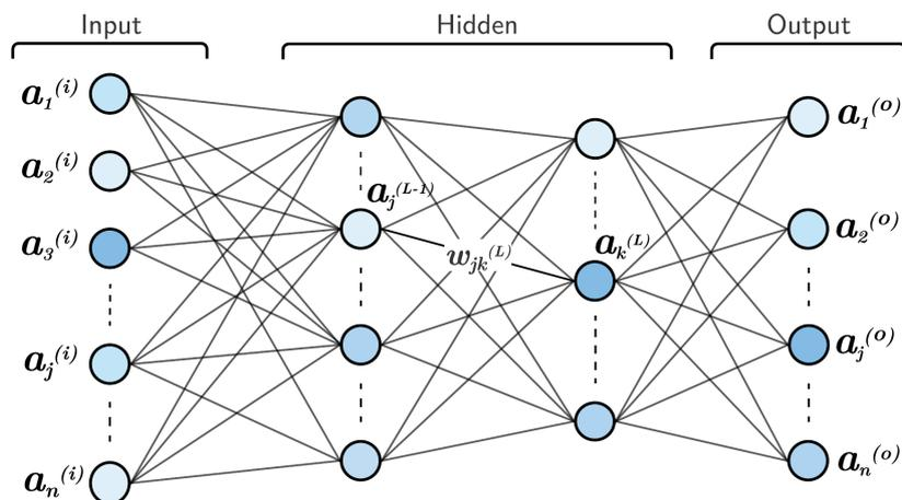
**Figure 3.3:** Simple Neural Net scheme. The input, output and hidden layers are put in evidence. Each neuron holds a value  $a_j^{(L)}$  and a bias  $b_j^{(L)}$ , while each connection holds a weight  $w_{jk}^{(L)}$ . The colours represent fictitiously the higher or lower value of the neurons.
