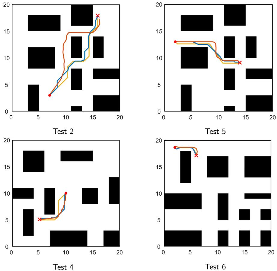
**Figure 6.3:** Comparison of the trajectories computed by the path planning algorithms. Orange lines represents RL trajectories, blue ones are A\* trajectories, and yellow ones are APF trajectories.
