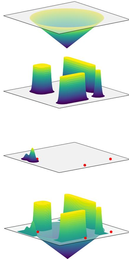
**Figure 4.3:** Layers forming the environment model used in the APF algorithm. The bottom one is the final environment model, corresponding to the sum of all the ones above.
