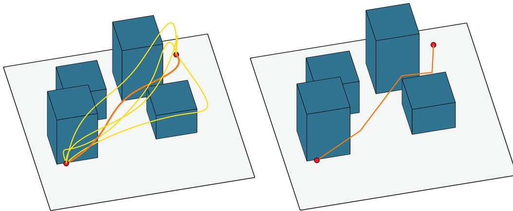
**Figure 2.1:** Comparison between a path generated with an heuristic path planning i.e. PSO algorithm on the left and a trajectory generated with the potential field approach on the right.
