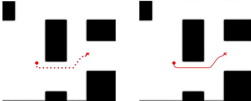
**Figure 4.13:** Interpolation of a series of points computed by the path planning agent.
