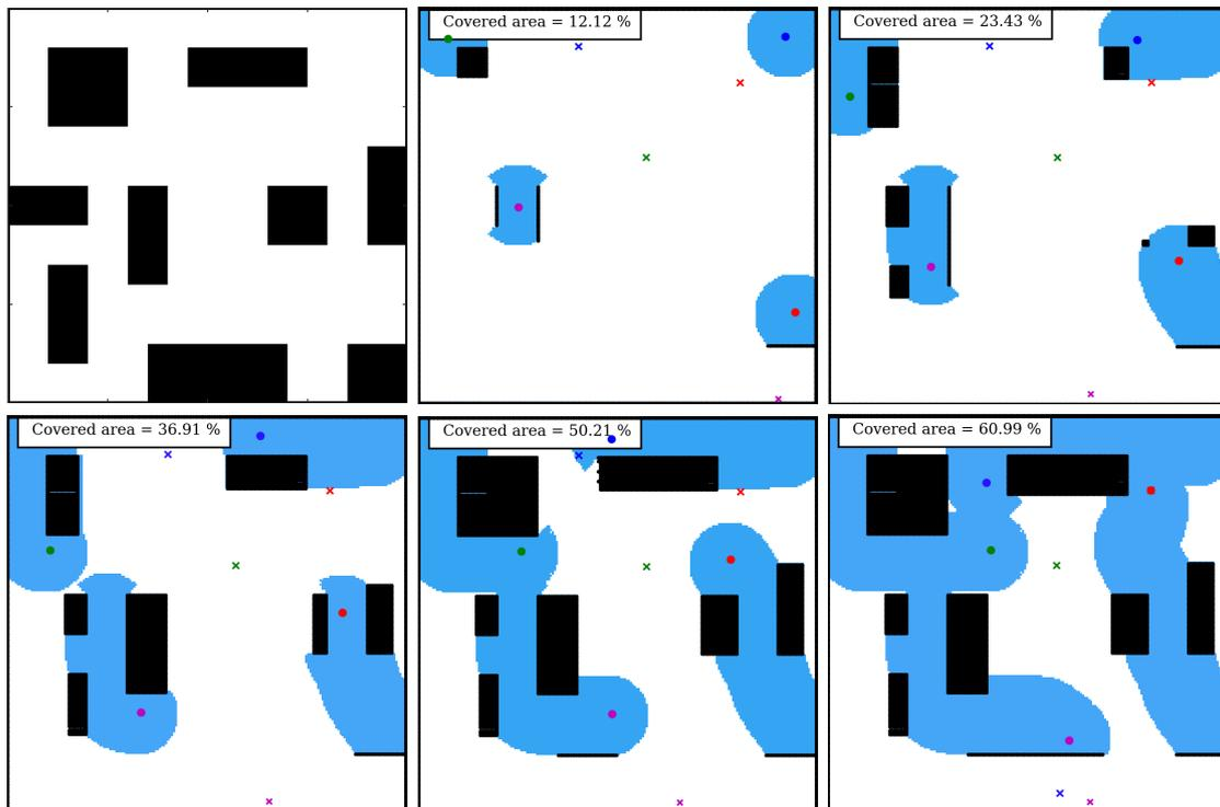
**Figure 6.6:** Simulation of the exploration task using the RL agent + k-means algorithm.
