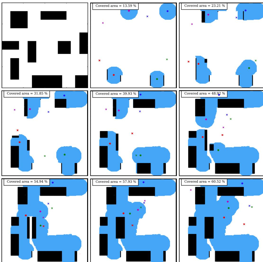
**Figure 6.8:** Simulation of the exploration task using k-means coverage algorithm.
