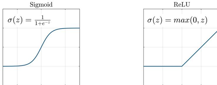
**Figure A.2:** Common choices for the activation functions. On the left the sigmoid activation function, whereas on the right the ReLU.
