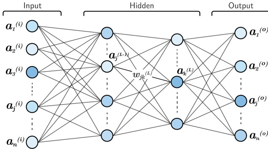
**Figure A.1:** Simple Neural Network scheme. Input, output and hidden layers are put in evidence. In general, any number of hidden layers can be used (copy of Figure 3.3).
