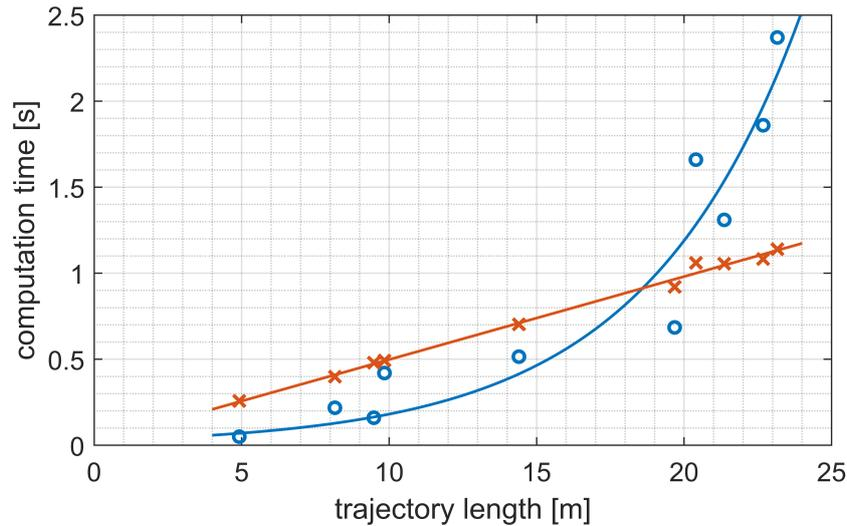
**Figure 6.4:** Comparison of the computational time<sup>25</sup> required by the RL agent (orange line) and  $A^*$  (blue line) to obtain trajectories of various lengths.
