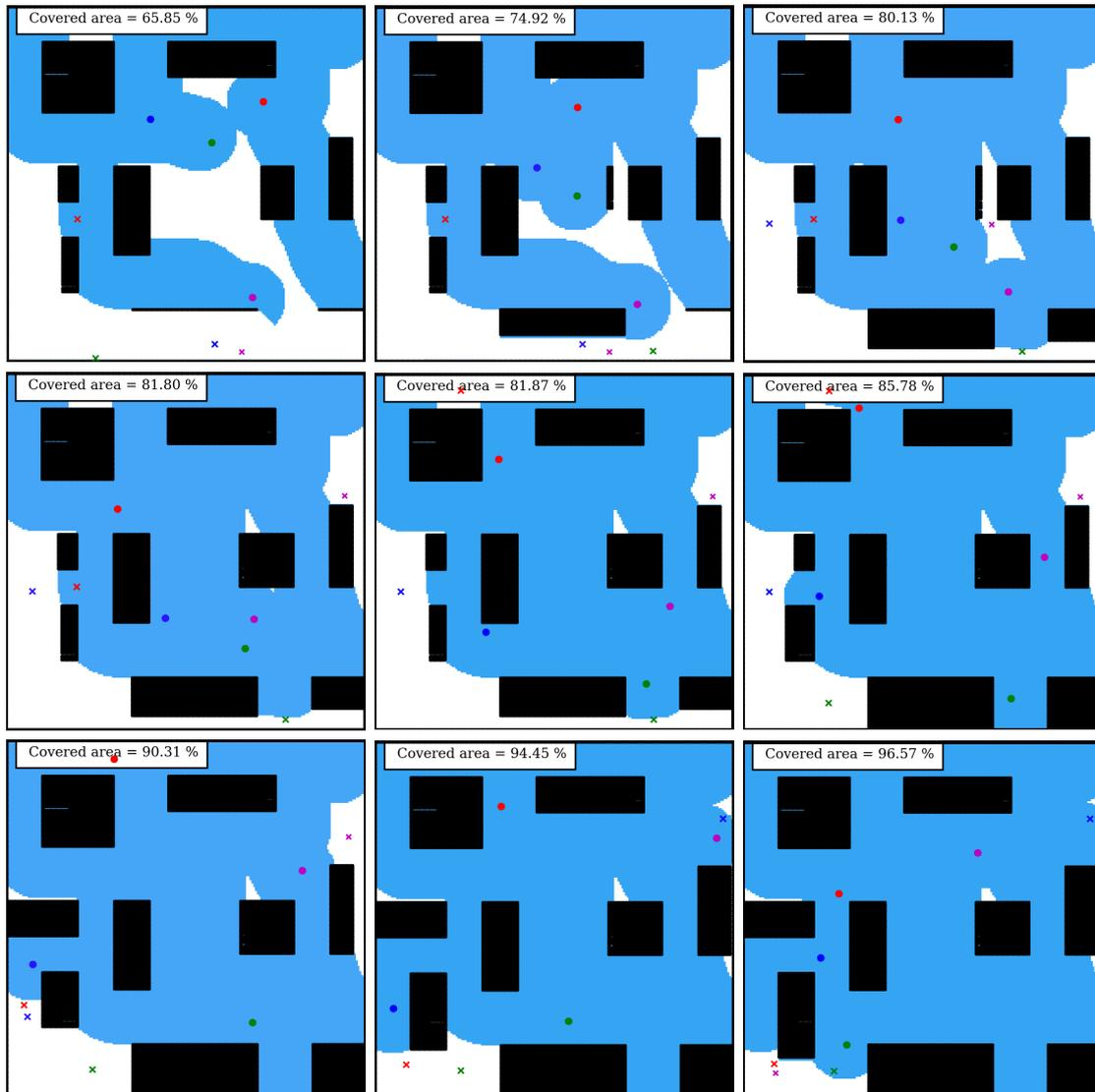
**Figure 6.7:** Simulation of the exploration task using the RL agent + k-means algorithm (pt 2).
