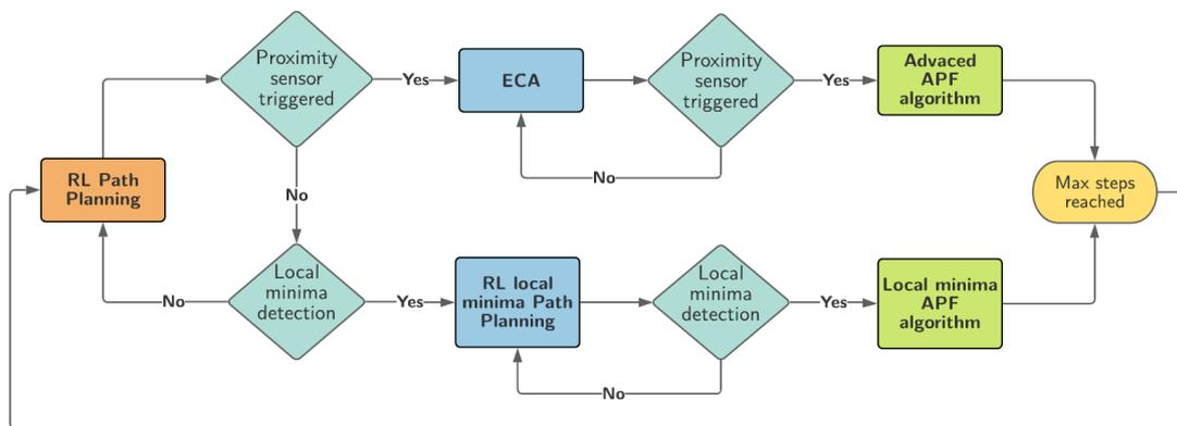
Figure 4.14: Logic diagram of the path planning algorithm.
