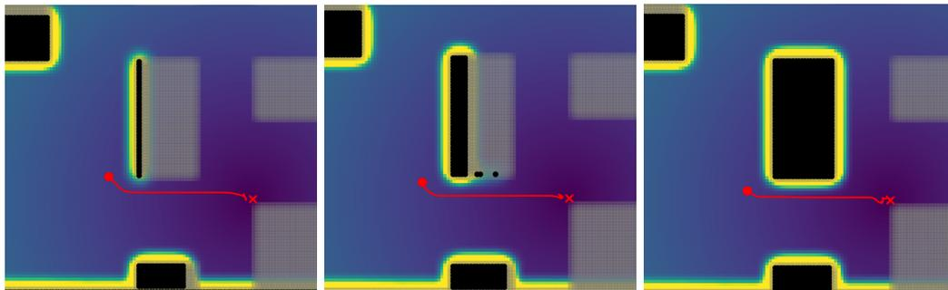
**Figure 4.6:** Detection and prediction of the full shape of an obstacle in the environment model builder. The grey areas are the unexplored obstacles whereas the black ones are the already explored obstacles. In the leftmost image the obstacle is identified as a wall whereas in the rightmost image the full shape of the obstacle is revealed.
