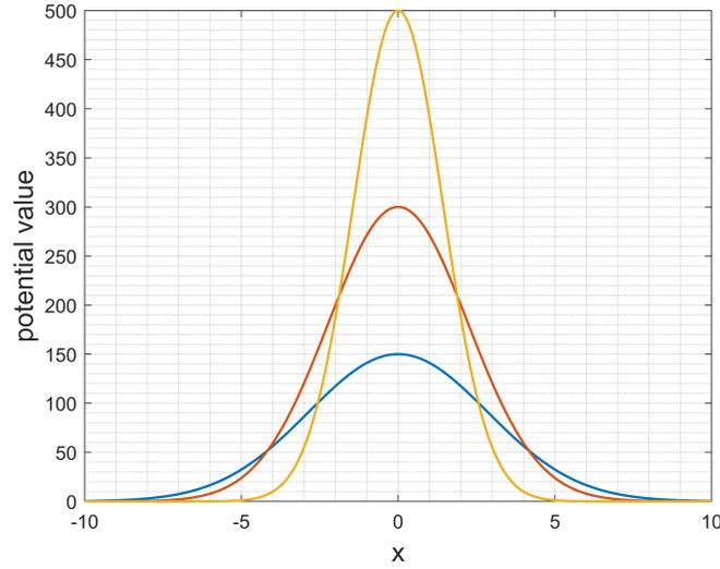
**Figure 4.8:** Distribution of the potential value within the obstacle matrix seen from a one dimensional point of view. Different distributions with disparate peak values are indicated.
