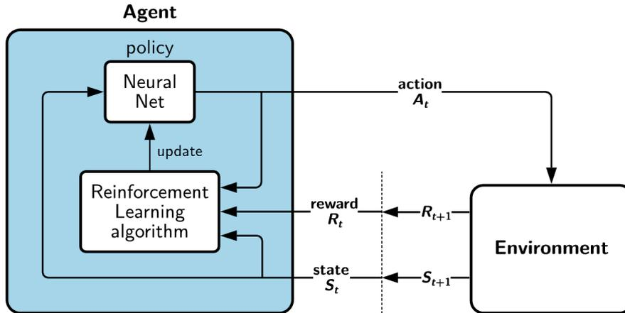
**Figure 3.4:** Block scheme representation of a RL training process. The basic structure is the same of the MDP represented in figure 3.2. However, in this case the agent internal structure and the presence of the RL training algorithm are put in evidence.
