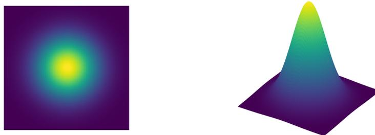
**Figure 4.7:** Matrix with a Gaussian distribution used for obstacle avoidance. The higher values of the matrix are visualised with the yellowest colour and they are the value associated with the highest risk (in this case the centre is the obstacle position.)
