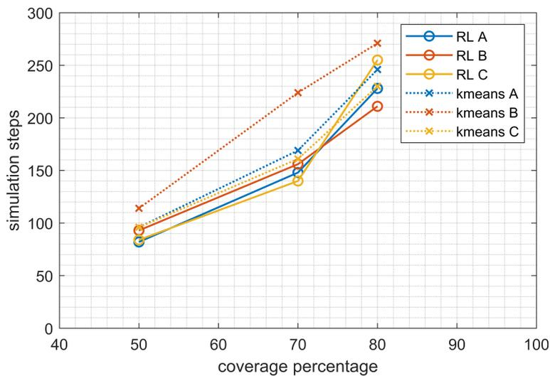
**Figure 6.10:** Comparison of the time employed to reach some coverage percentage thresholds in the six exploration tests.
