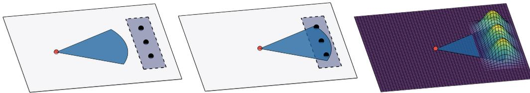
**Figure 4.4:** Obstacle detection and creation procedure in the the environment model builder. In the leftmost image, the obstacles (black dots) are out of vision range. In the image in the middle obstacles are detected. In the rightmost image the potential is raised around the newly discovered obstacles.
