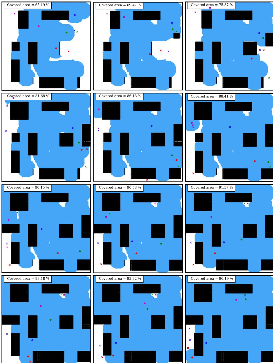
**Figure 6.9:** Simulation of the exploration task using k-means coverage algorithm (pt 2).
