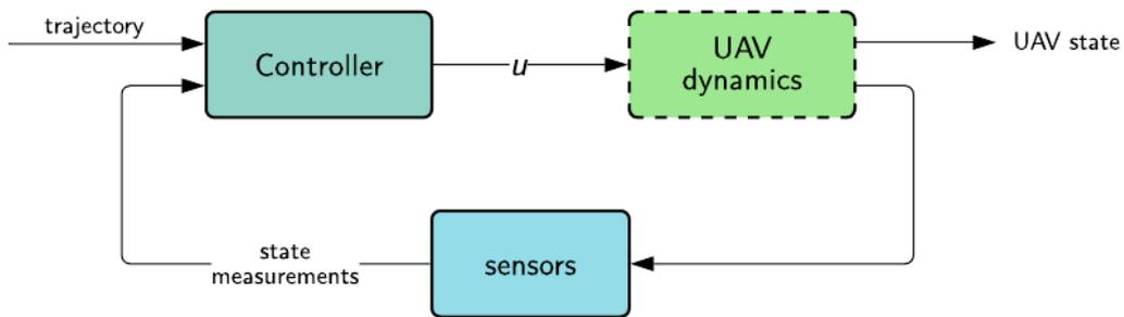
**Figure 4.15:** Block scheme of the control loop algorithm.
