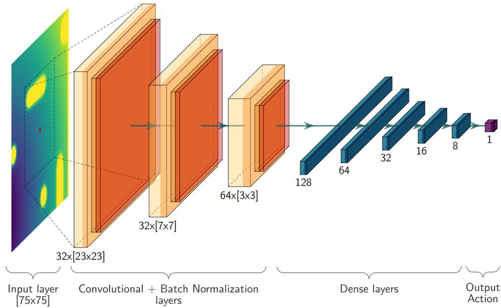
**Figure 4.12:** Neural net of the actor used in the path planning. The input of the neural net is a portion of the potential map around the drone and after the convolutional and dense part the output is obtained as the direction to follow.
