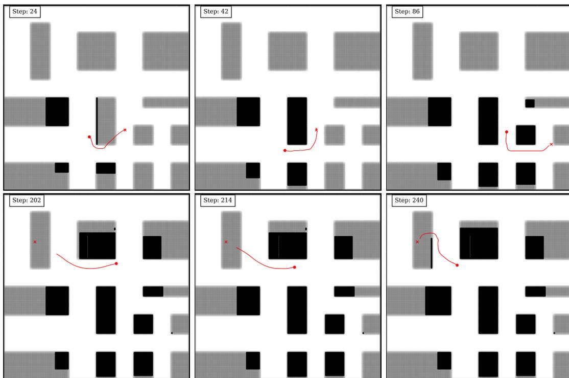
**Figure 6.2:** Simulation of Path Planning agent in validation map C.
