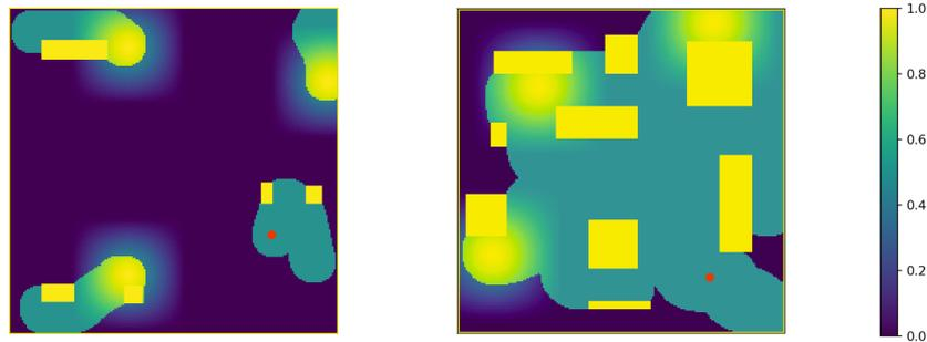
**Figure 4.9:** Example of two Coverage agent input states. The matrices displayed have dimension  $[200 \times 200]$ , representing an environment of size  $[20m \times 20m]$  with a resolution of 0.1m. The colour bar shows the value of each point.
