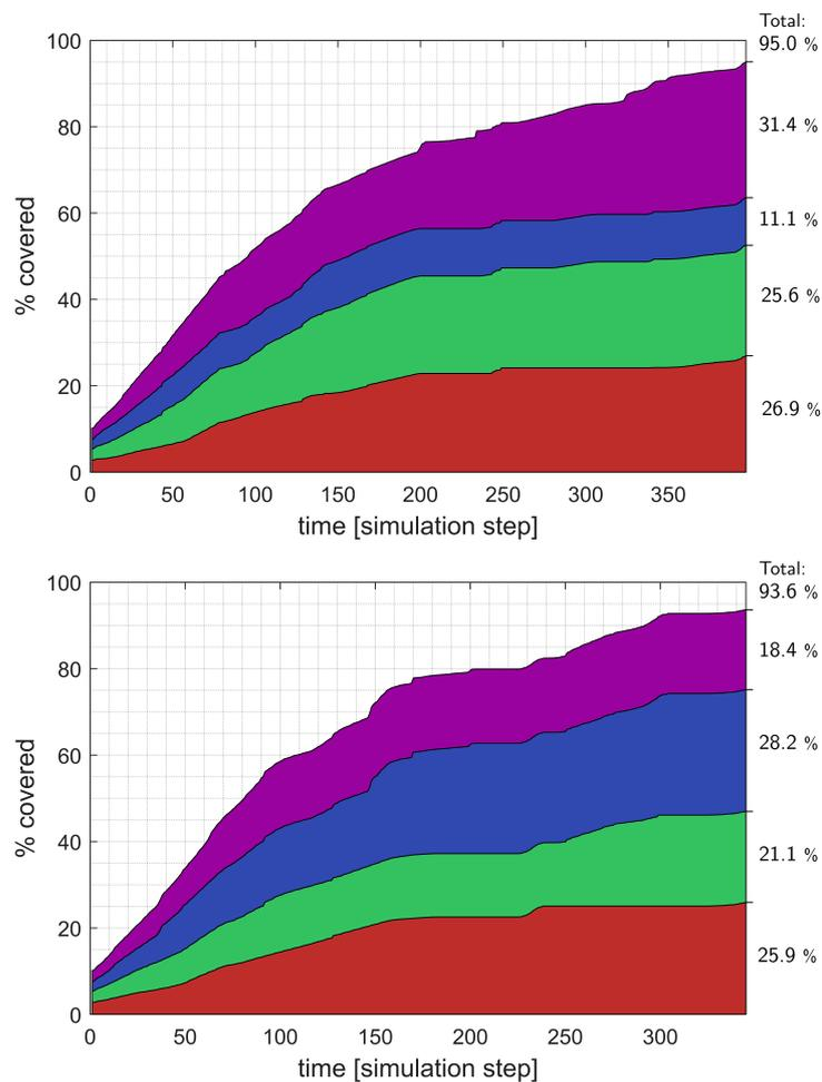
**Figure 6.11:** Coverage percentage of the single UAV contributions in the exploration process for tests 1 and 4. The plot on the top shows the results of test 1, whereas the one on the bottom shows results of test 4. The colours correspond to those of the UAVs represented in the simulations of figures 6.8, 6.9, 6.6, and 6.7.
