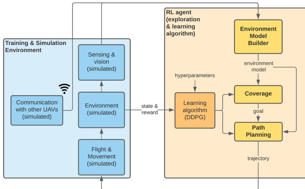
**Figure 4.1:** Block diagram of the learning process. The yellow blocks are the two RL agents and the learning algorithm, whereas the blue ones are the parts used for the environment simulation in the training process.
