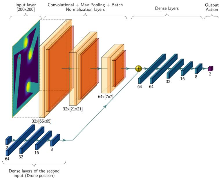
**Figure 4.10:** Representation of the neural network structure of the Coverage actor.<sup>14</sup>
