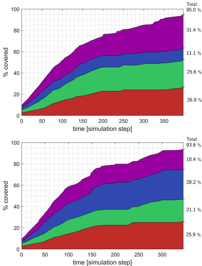
**Figure 6.12:** Coverage percentage of the single UAV contributions in the exploration process for tests 1 and 4. The plot on the top shows the results of test 1, obtained in map A using the only k-means coverage algorithm. The one on the bottom shows results of test 4, which is performed using the combined coverage agent. The colours correspond to those of the UAVs represented in the simulations of figures 6.9, 6.10, 6.7, and 6.8.
