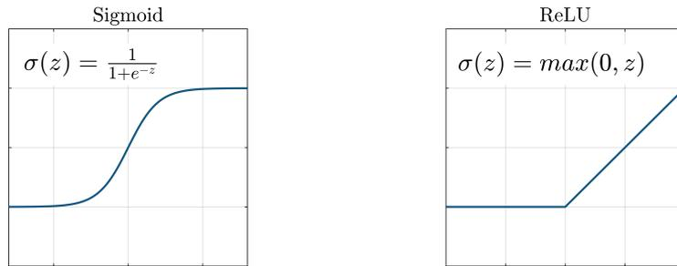
**Figure A.2:** On the left, the sigmoid activation function. On the right, the ReLU.
