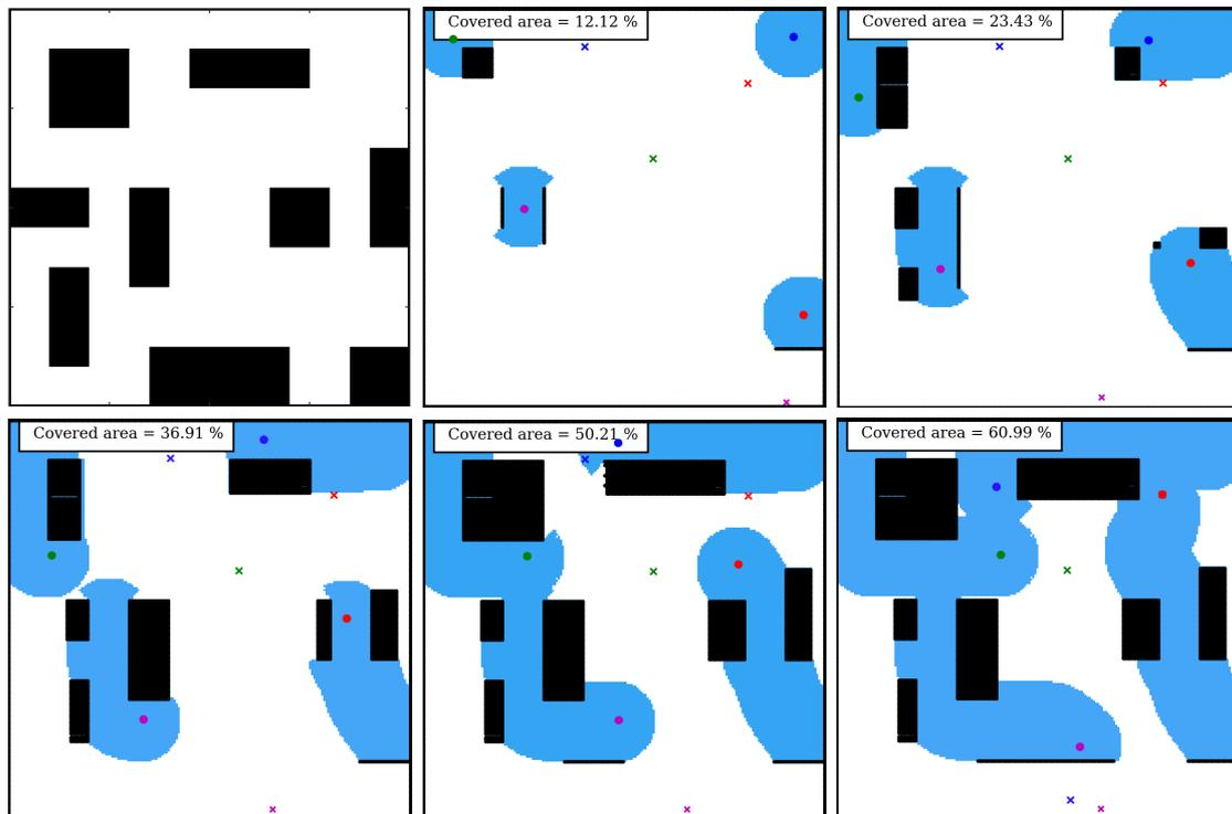
Figure 6.7: Exploration simulation using the RL agent + k-means coverage algorithm.
