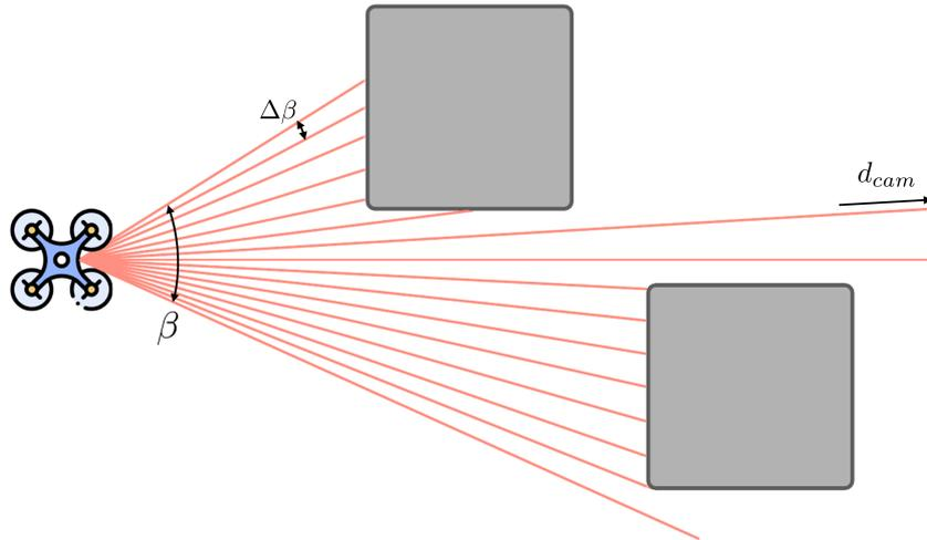
**Figure 4.8:** Implementation of the vision function using a simulated depth camera.
