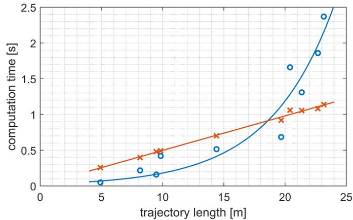
**Figure 6.6:** Comparison of the computational time required by the RL agent (orange line) and A\* (blue line) to obtain trajectories of various lengths.
