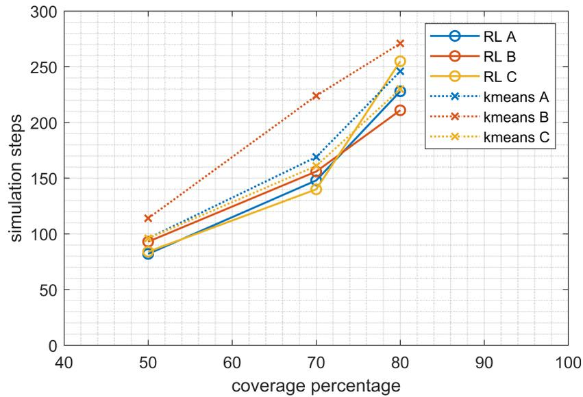
**Figure 6.11:** Comparison of the time employed to reach some coverage percentage thresholds in the six exploration tests.
