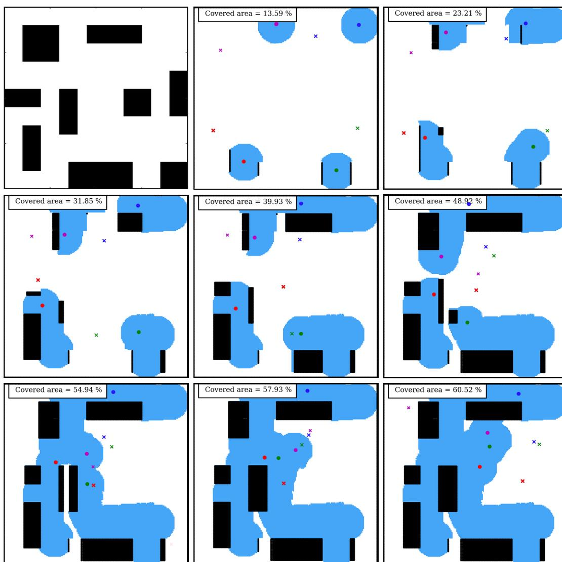
Figure 6.9: Exploration simulation using the k-means coverage algorithm.
