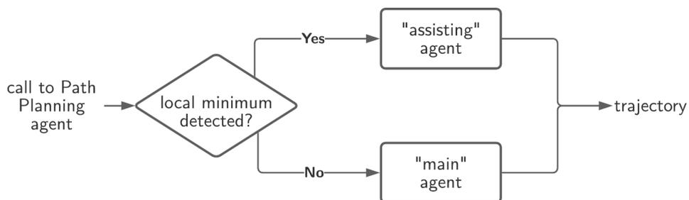
**Figure 6.4:** Logical flow through which the right path planning agent is selected to compute the trajectory every time the path planning routine is called. Both the agents use the routine of algorithm 4.2 to compute the path.
