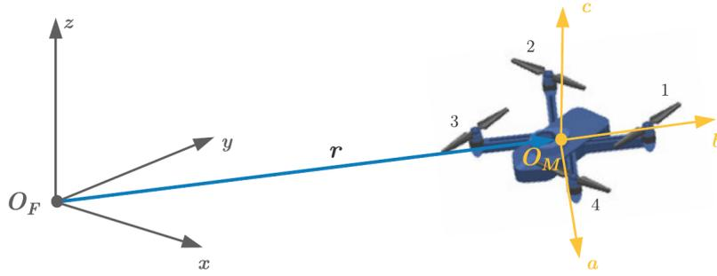
**Figure 4.17:** Reference frames used to build the UAV dynamic model
