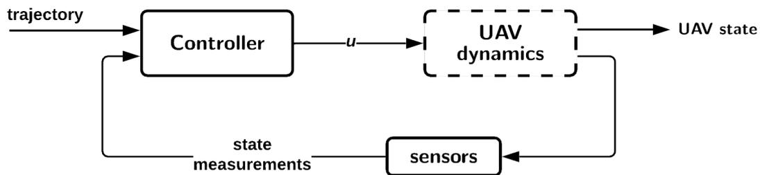
Figure 4.18: Block scheme of the control loop algorithm.
