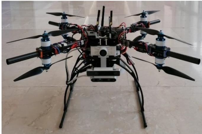
**Figure 4.16:** The DRAFT team quadcopter that has been used as reference.
