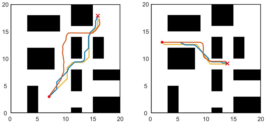
**Figure 6.5:** Comparison of the trajectories computed by the path planning algorithms in test 2 (on the left) and test 5 (on the right). Orange line represents RL trajectory, blue is A\*, and yellow is APF.
