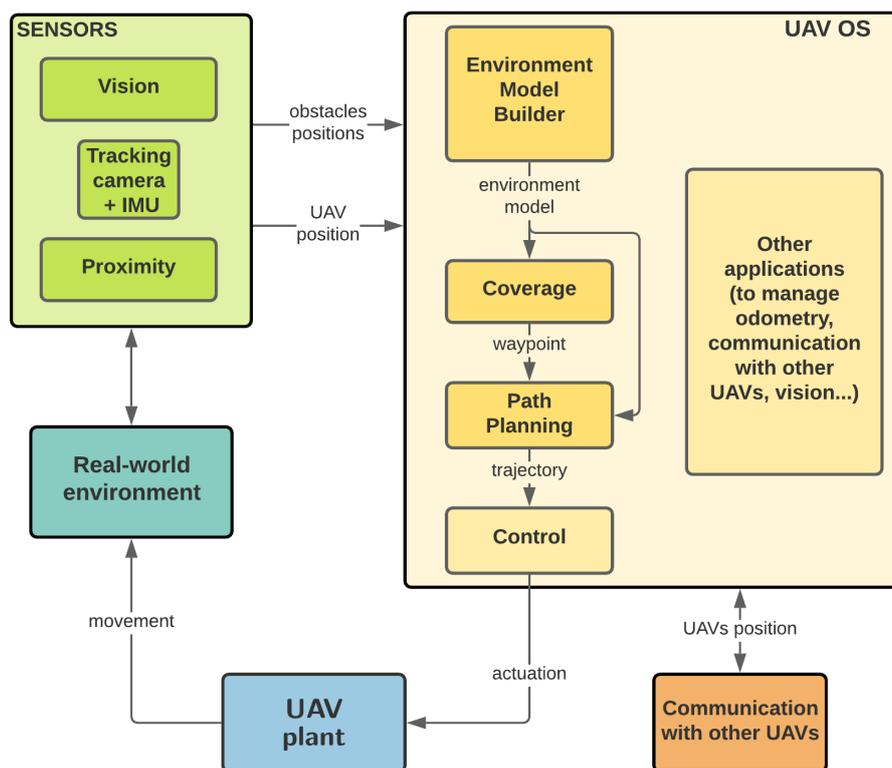
**Figure 4.3:** Block scheme of the algorithm structure deployed for a real-world application. The light-yellow block represents the UAV OS and contains the proposed algorithm. The UAV and the blocks representing the real-world, have to be treated as black boxes, and can be interacted with only through the actuation of the UAVs motors or through sensors.
