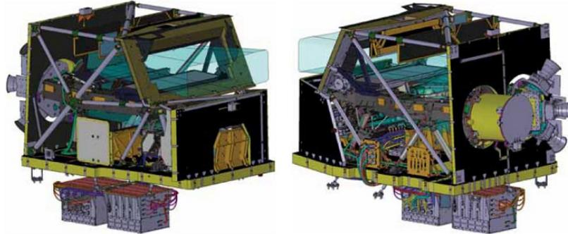
**Figure 1.2:** Sentinel-2 Multispectral Instrument produced by Airbus Defence and Space). Source: ESA
