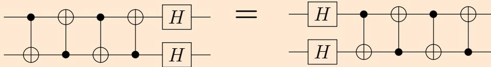
Figure 2.29: Examples of template application through a cluster of “alternated” CX gates, with H gates moved backwards
