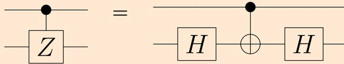
Figure 3.2: Template to transform a CZ gate into a CX gate through the insertion of H gates
