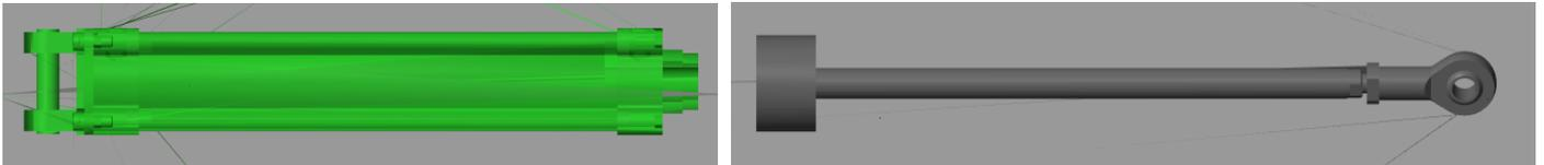
Figure 4.80: The bigger cylinder used with the backframe (2 cylinders used) (colors are only for visualization).
