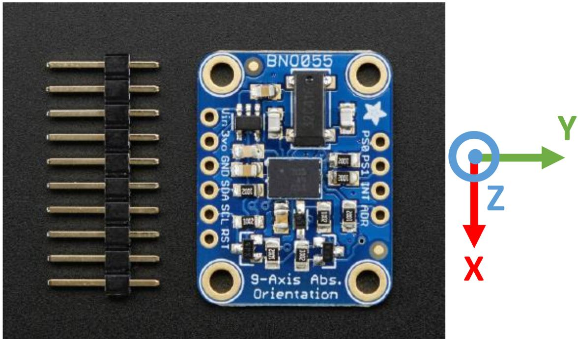
Figure 3.45: Adafruit BNO055 absolute orientation sensor (Appendix J).
