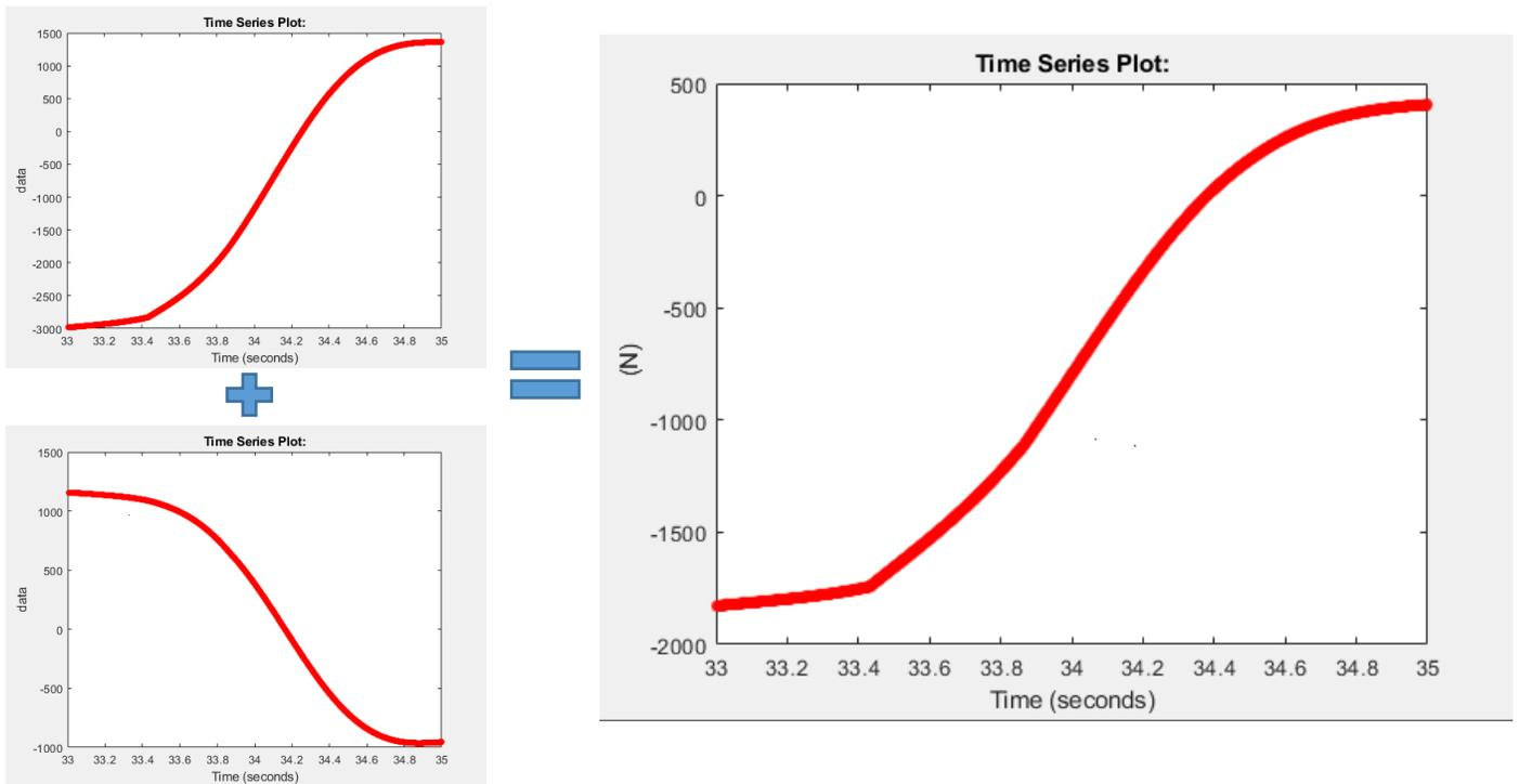
Figure 4.99: Summation of the lower back cylinder forces in fourth state and the final force required from this cylinder at this state (Forces in N).
