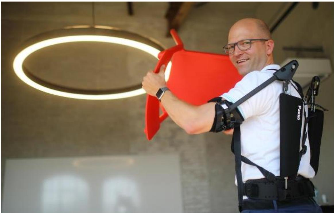
*Figure 1.11: Ottobock Paexo Upper extremity exoskeleton.*
