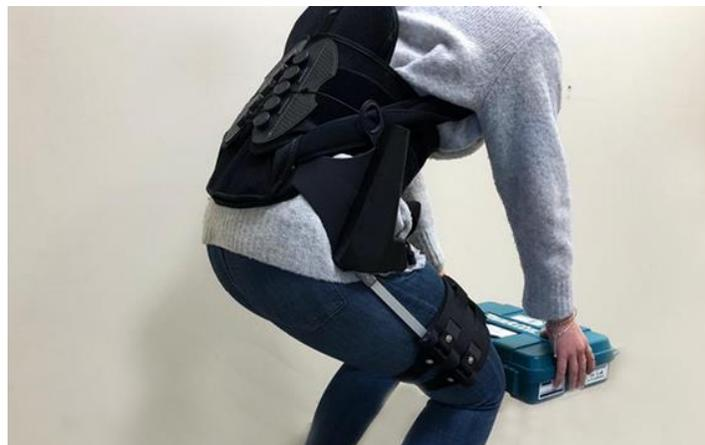
*Figure 1.15: Passive type exoskeleton.*
