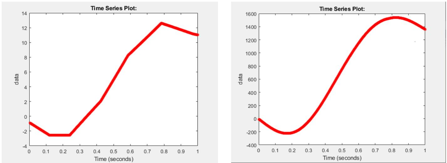
Figure 4.91: Left: upper cylinder force (N), Right: lower cylinder force (N).
