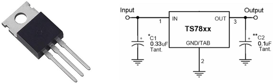
Figure 3.50: TS7812 Voltage regulator and pinout
