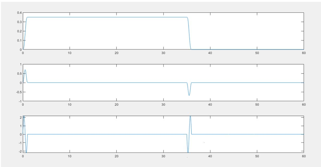
Figure 3.84: Kinematics of the hip joint. (x-axis is in s) (y-axis is in rad, rad/s and rad/s/s).
