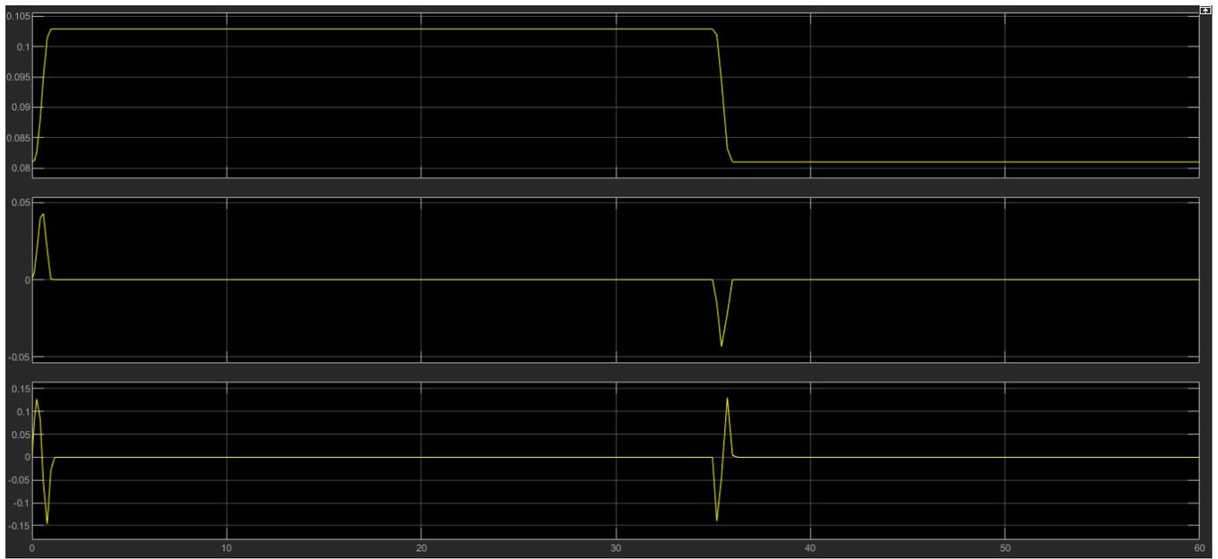
Figure 4.88: Kinematics of the small lower cylinder. (x- axis is in s) (y-axis is in m, m/s and m/s/s).
