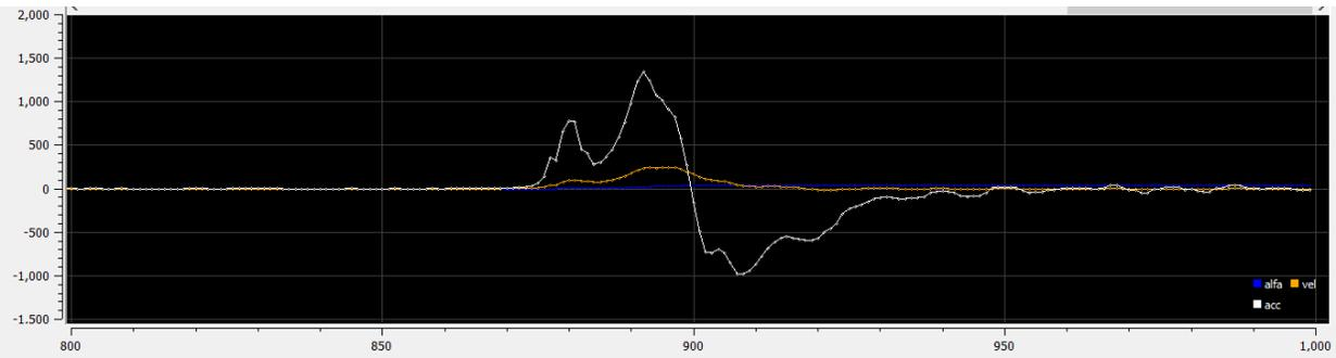
Figure 3.73: Measurement of the angular velocity (yellow) in counterclockwise rotation (x-axis is time in ms, and y-axis is angle rate in rad/s) with weights filter.
