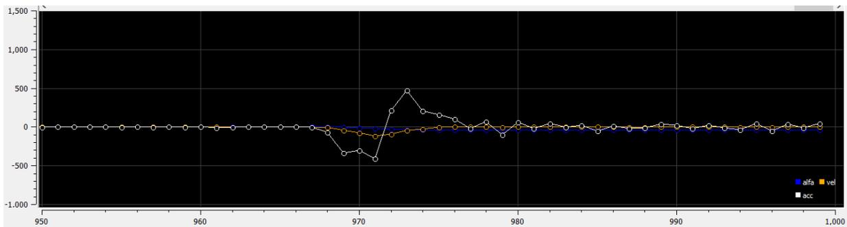
Figure 3.71: Measurement of the angular acceleration (white) in clockwise rotation (x-axis is time in ms, and y-axis is velocity rate in  $\text{rad/s}^2$ ) with delay filter.
