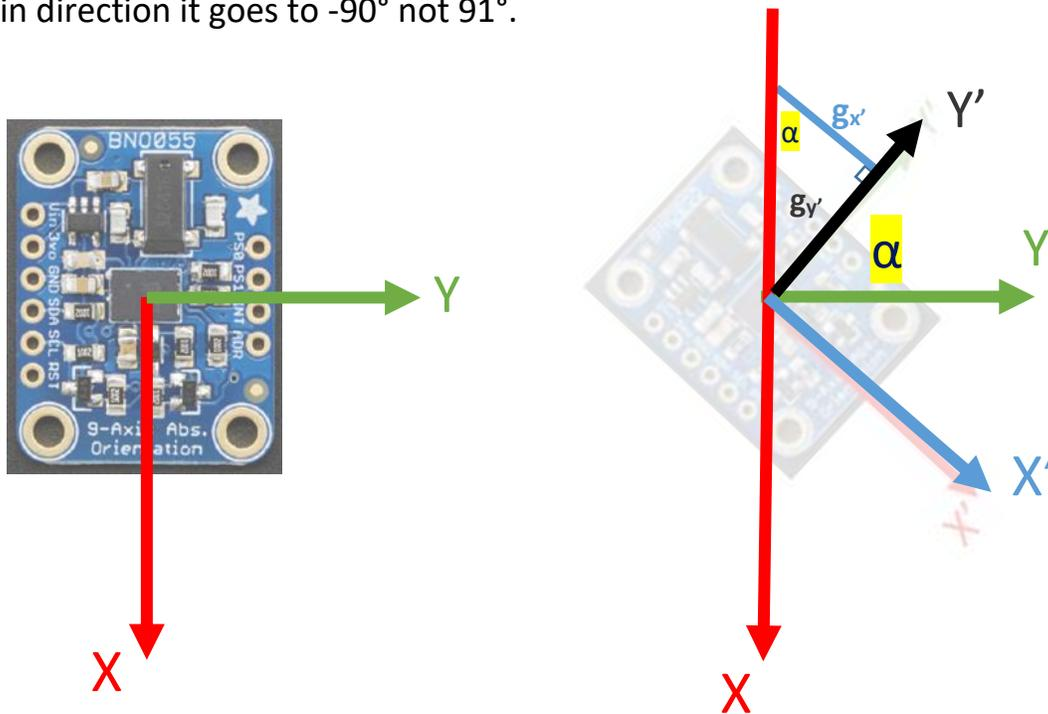
Figure 3.59: Counterclockwise graphical orientation of the sensor.
