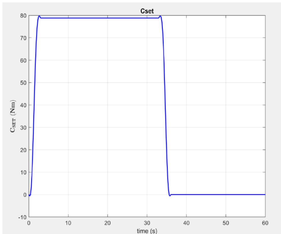
Figure 2.20:  $C_{SET}$  value of the torque that is 30% of the human torque.
