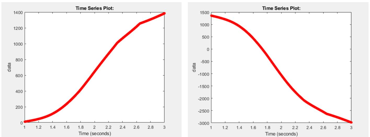
Figure 4.93: Left: upper cylinder force (N), Right: lower cylinder force (N).
