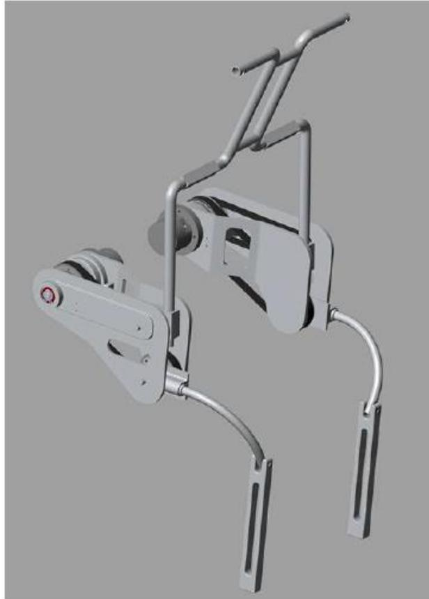
*Figure 2.33: Complete model of exoskeleton on Simscape after assembly.*
