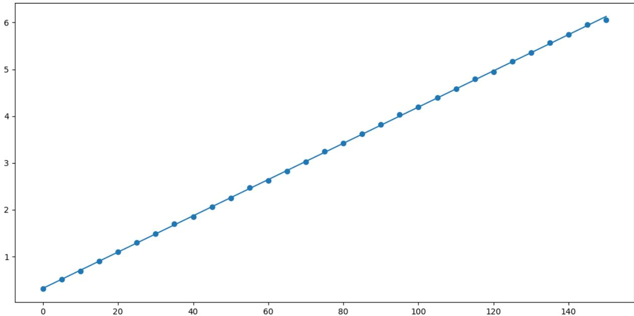
Figure 3.55: Python linear regression output (x-axis is Arduino code data; y-axis is valve Pressure).
