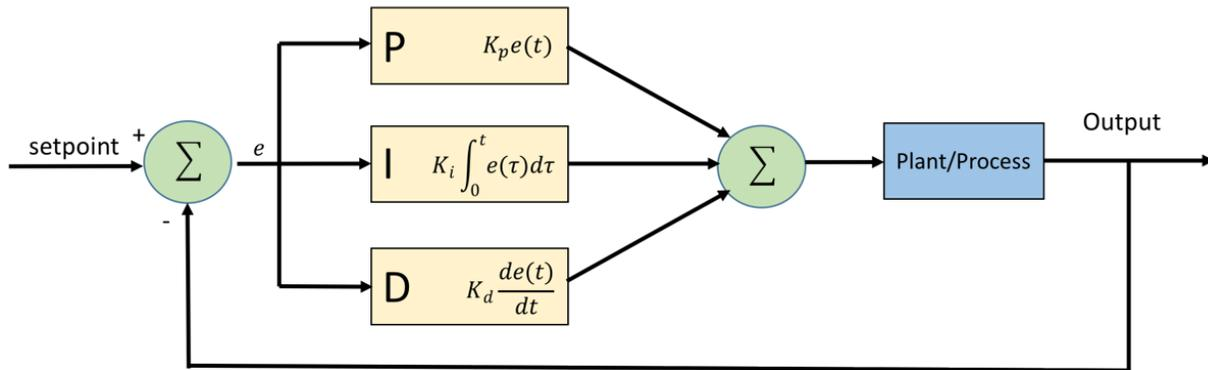
Figure 2.26: Schematic of a PID controller.
