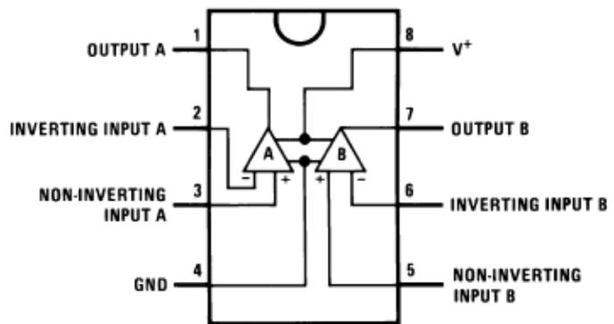
Figure: 3.49: LM358-n operational amplifier and the pinout data.
