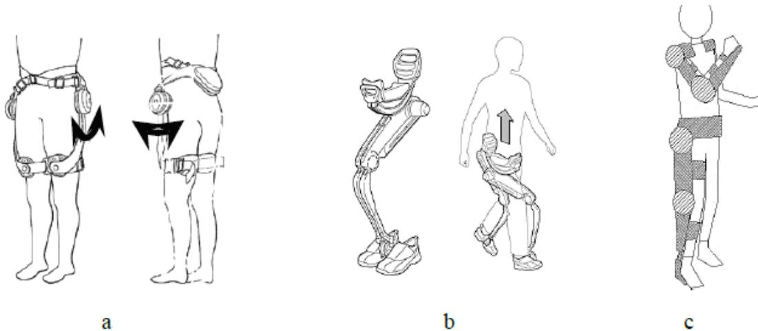
Figure 1.8B: Basic exoskeleton designs shown in ISO 13482 (a) Leg motion assistive device, (b) Body weight supportive device, (c) Exoskeleton wearable robot.
