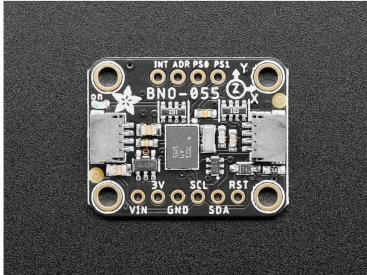
The new version of the board includes [SparkFun qwiic \(https://adafru.it/Fpw\)](https://adafru.it/Fpw) compatible [STEMMA QT \(https://adafru.it/Ft4\)](https://adafru.it/Ft4) connectors for the I2C bus so you don't even need to solder! Use a plug-and-play STEMMA QT cable to get 9 DoF data ASAP.
