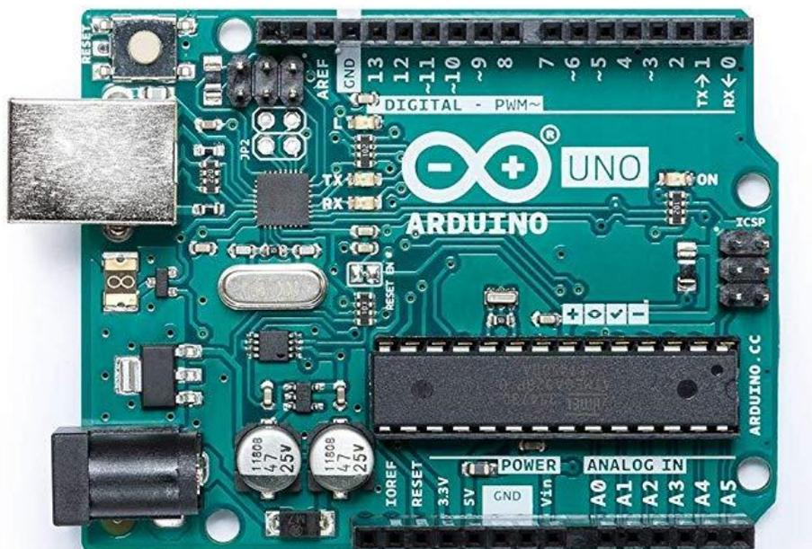
*Figure 3.41: Arduino UNO (Appendix I), one of the most common Arduino boards.*
