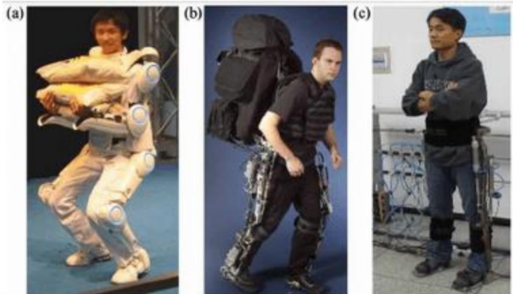
*Figure 1.6: Walking assistive exoskeleton: (a) HAL-5 system [16]; (b) BLEEX lower limb exoskeleton [17]; (c) exoskeleton leg for human's walking power augmentation of Zhejiang University*
