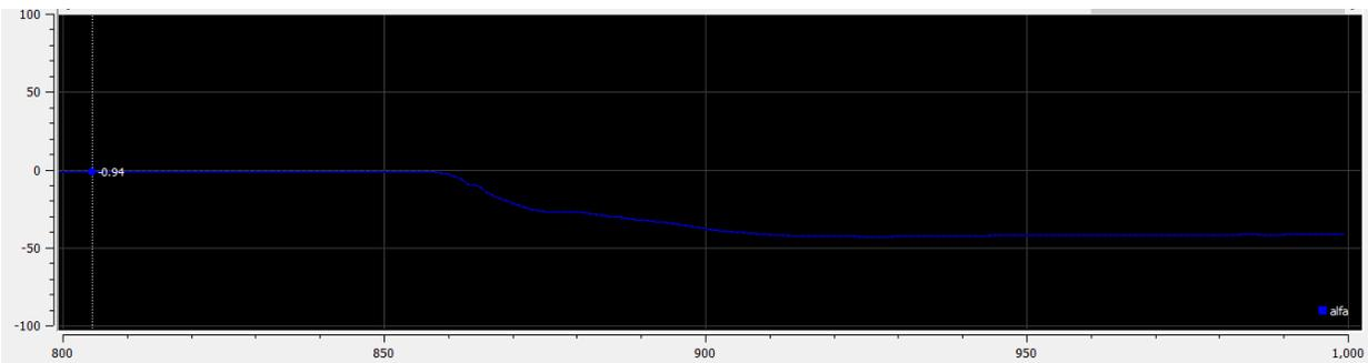
Figure 3.63: Measurement of the angular position (blue) in clockwise rotation (x-axis is time in ms, and y-axis is angle in degrees).
