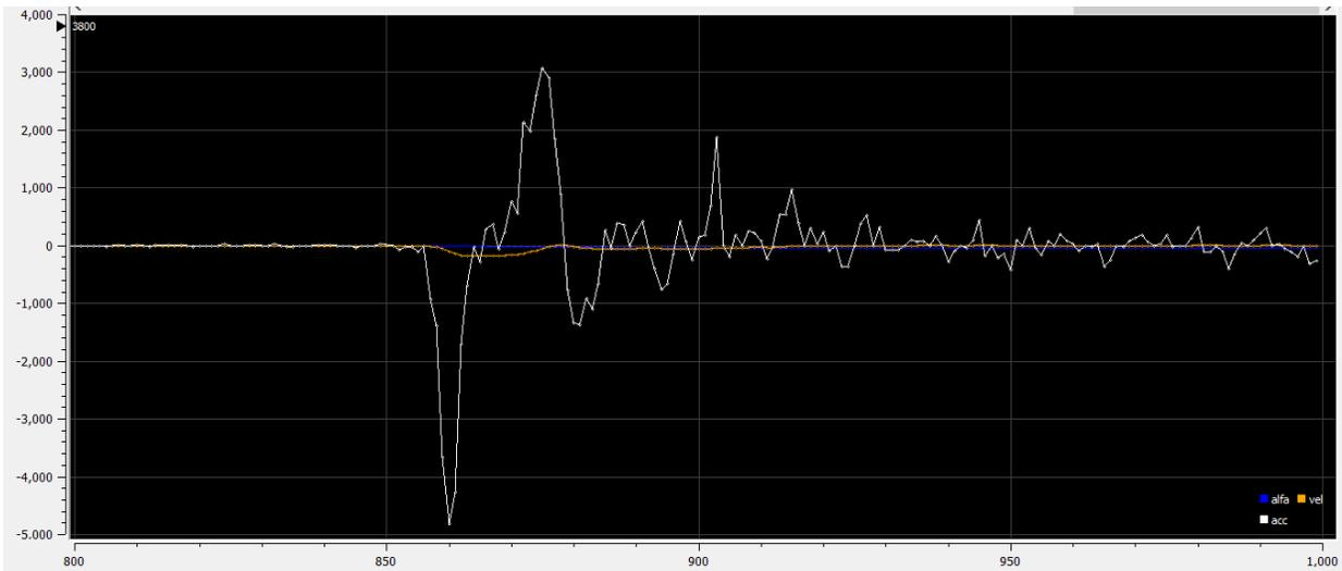
Figure 3.65: Measurement of the angular acceleration (white) in clockwise rotation (x-axis is time in ms, and y-axis is velocity rate in  $\text{rad/s}^2$ ).
