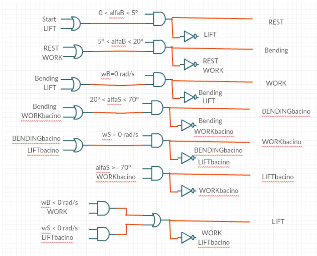
Figure 3.58: logical control representing the states of operation.
