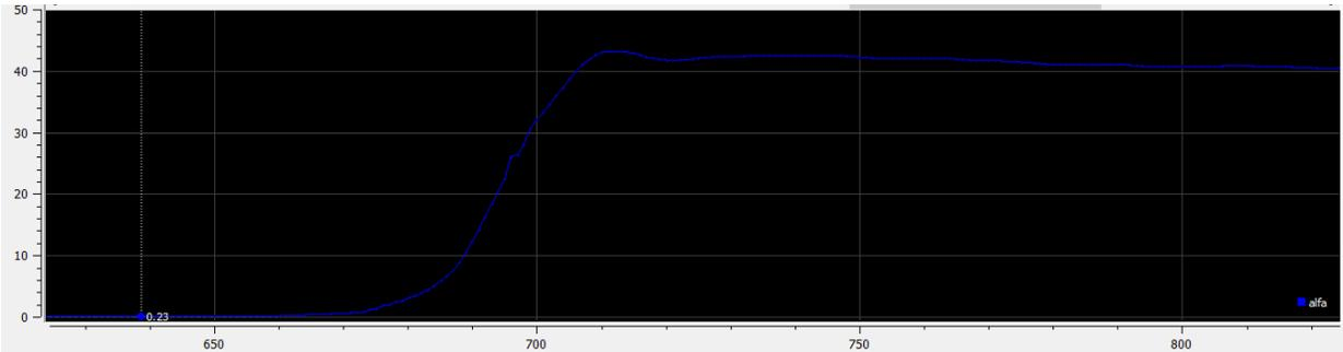
Figure 3.60: Measurement of the angular position (blue) in counterclockwise rotation (x-axis is time in ms, and y-axis is angle in degrees).
