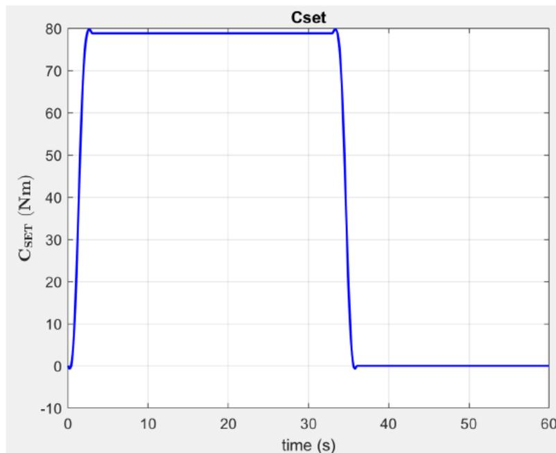
Figure 2.27: Reference Torque.
