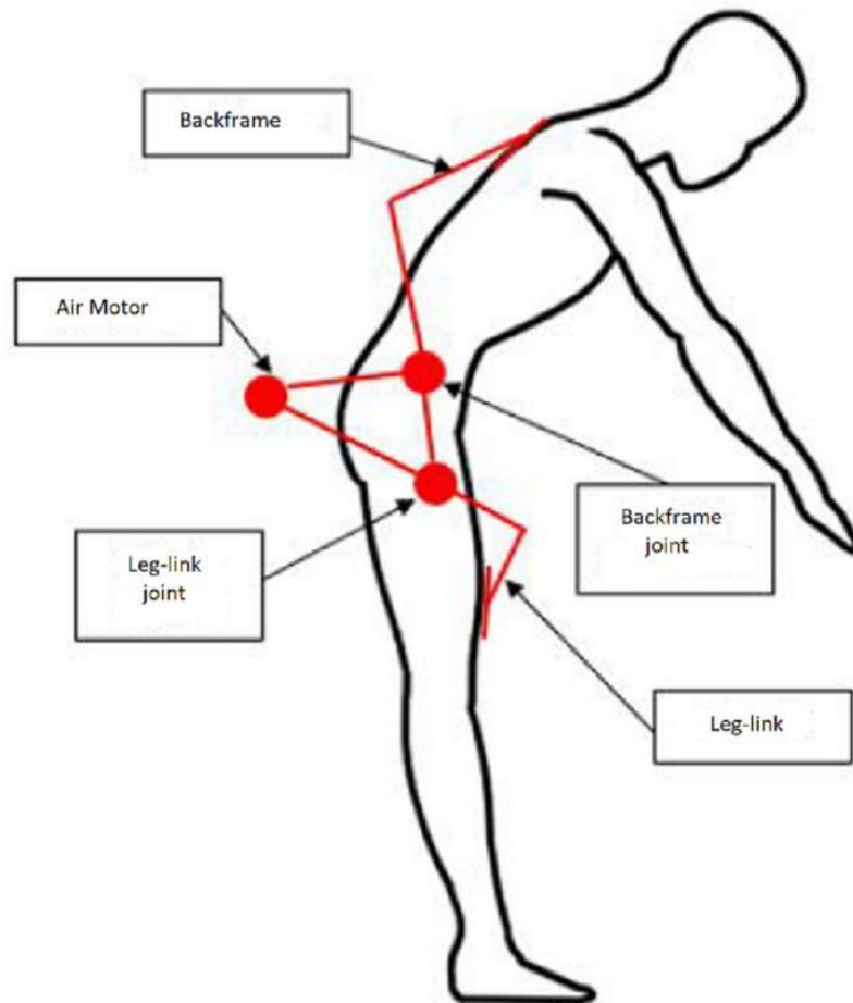
*Figure 1.17: Design concept of the pneumatic exoskeleton.*
