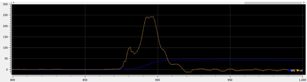
Figure 3.74: Measurement of the angular acceleration (white) in counterclockwise rotation (x-axis is time in ms, and y-axis is velocity rate in  $\text{rad/s}^2$ ) with weights filter.
