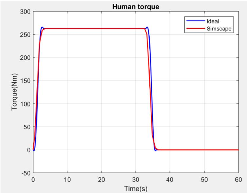
Figure: 2.37: Comparison between the torque generated by the formula and the one produced by the Simscape model.
