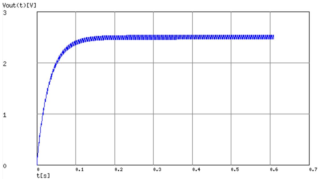
Figure 3.51: step response of 0-5 V PWM with 50% duty cycle.
