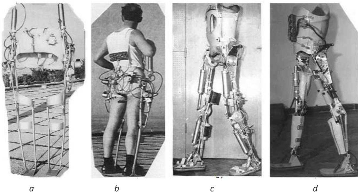
*Figure 1.4: World's first walking active exoskeleton (a and b); active exoskeleton for rehabilitation of paraplegics and similar disabled persons (c); Active exoskeleton with electromechanical drives (d).*
