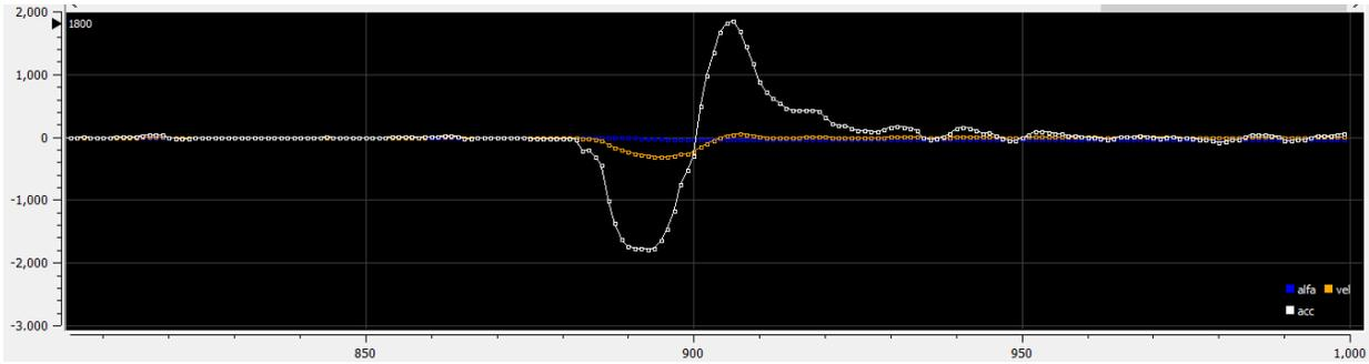
Figure 3.77: Measurement of the angular acceleration (white) in clockwise rotation (x-axis is time in ms, and y-axis is velocity rate in  $\text{rad/s}^2$ ) with weights filter.
