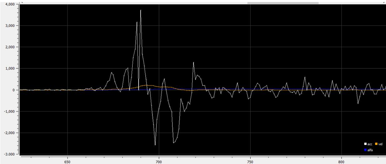
Figure 3.62: Measurement of the angular acceleration (white) in counterclockwise rotation (x-axis is time in ms, and y-axis is velocity rate in  $\text{rad/s}^2$ ).
