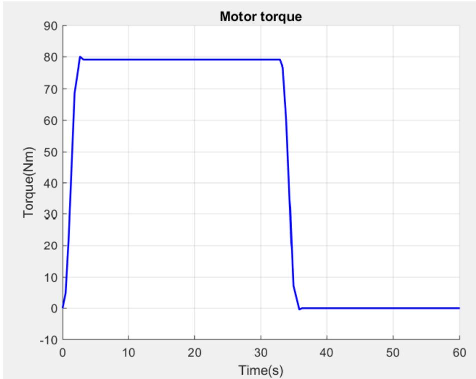
Figure 2.34: Torque produced by the imported Solidworks model.
