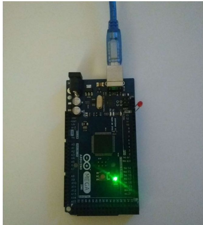
Figure 4-1: A LED connected to pin 13
