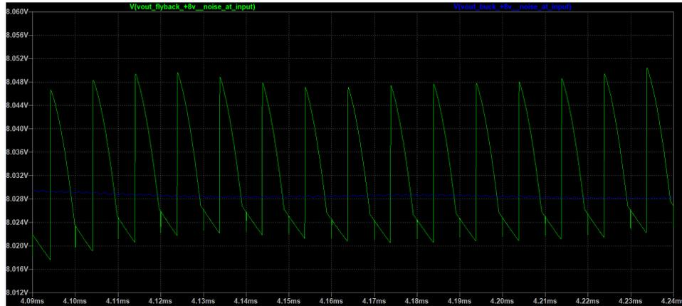
Figure 6.10: LT8613 and Custom Fly-back +8V output comparison with noise at the input at steady state.
