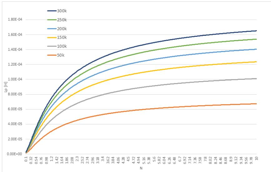
Figure 8.2: Primary Inductance value Vs Turn Ratio.
