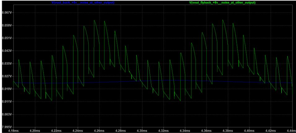
Figure 6.11: LT8613 and Custom Fly-back +8V output comparison with noise at the output +5V converter at steady state.
