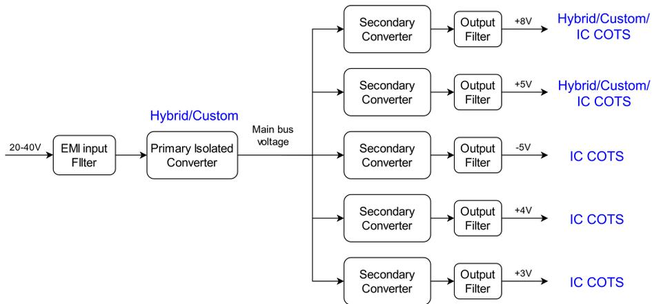
Figure 6.7: First architecture with Filter topology.
