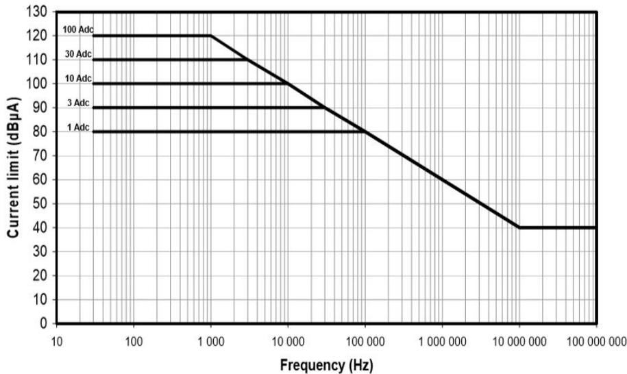
Figure 6.2: Conductive Susceptibility mask.
