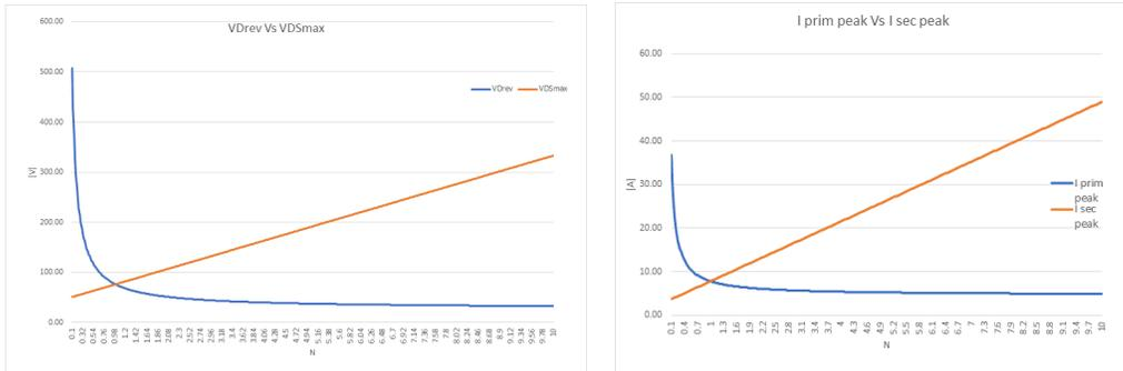
Figure 8.3: Diode and Drain-Source voltage, Primary and Secondary current Vs Turn Ratio.
