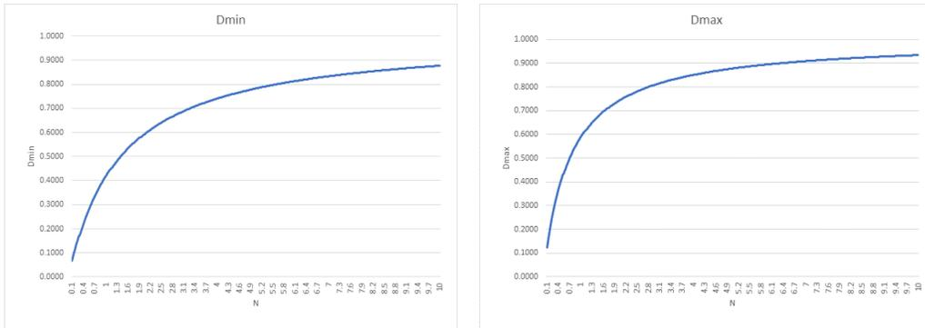
Figure 8.1: Minimum and Maximum Duty Cycle Vs Turn Ratio.
