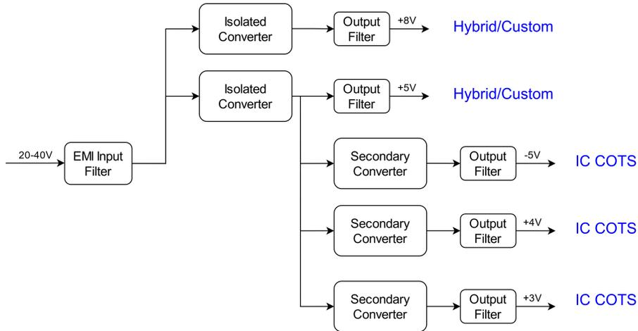
Figure 6.8: Second architecture with Filter topology.
