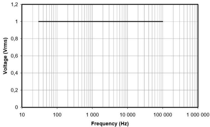
Figure 6.1: Conductive Emission mask.
