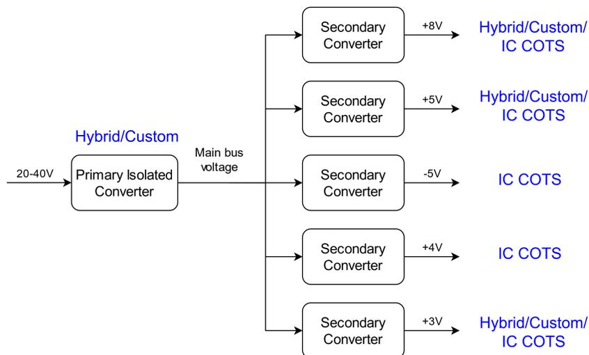
Figure 4.4: Combinations of converters for architecture 1.
