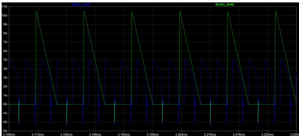
Figure 7.3: Secondary current for Fly-back in CCM and DCM.
