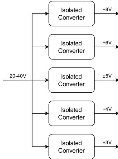
Figure 3.3: Multiple isolated architecture or Family 2
