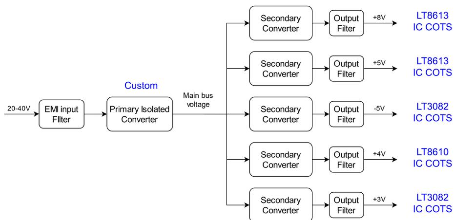
Figure 6.12: Final architecture of the PSM.
