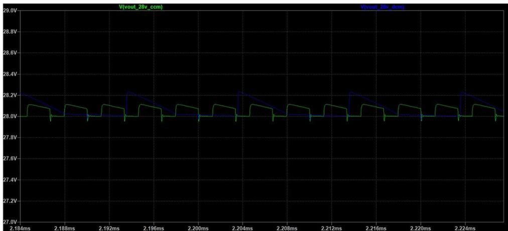
Figure 7.2: Output voltage for Fly-back in CCM and DCM.
