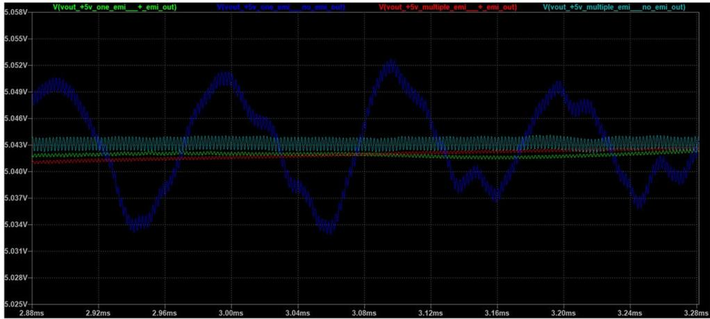
Figure 6.5: Output of LT8613 converter for different Filter topology.
