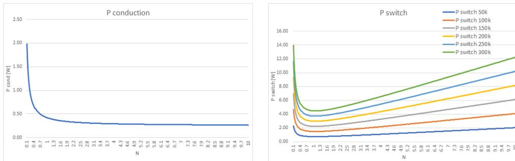
Figure 8.4: Conduction and Switching Losses Vs Turn Ratio.
