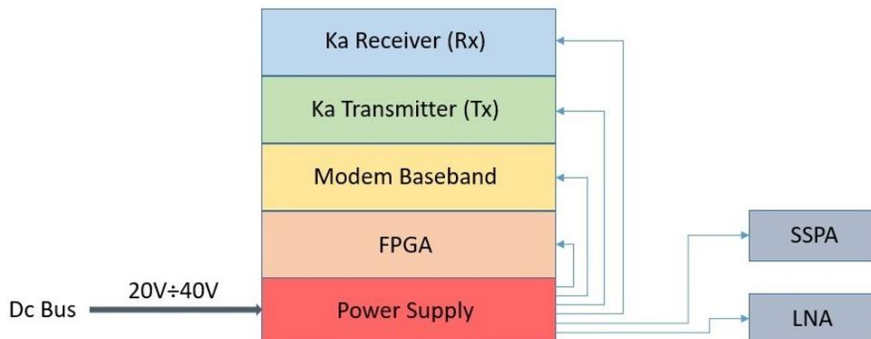
Figure 3.1: SDR, SSPA and LNA subsystem power connection
