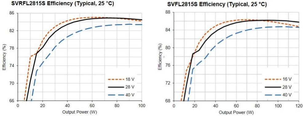
Figure 4.3: Efficiency over Power curves for SVRFL and SVFL [10] [11].
