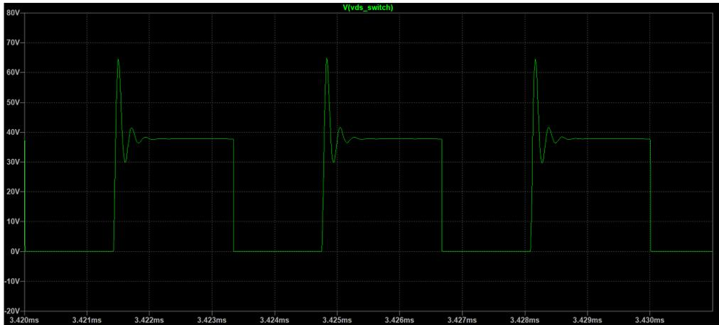
Figure 8.6: Voltage at the drain-source of the switch.
