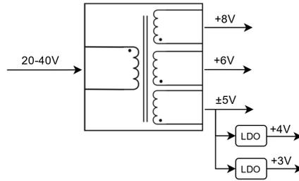
Figure 3.4: Fly-back multiple output architecture or Family 3
